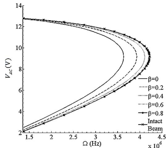
**Fig. 15. Suppression zone of the pull-in instability versus  $V_{DC}^2+V_{AC}^2/2=81.33$  and relative depth ratio  $n=0.1$  and different relative crack locations  $\beta$**
