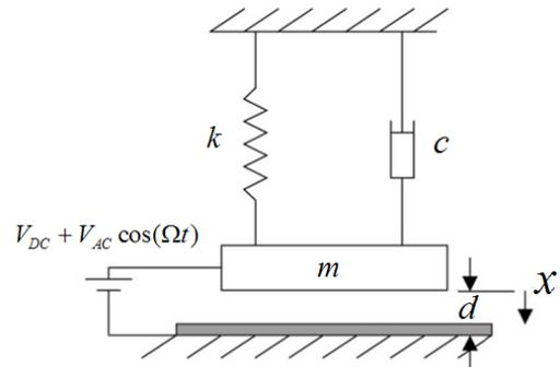
Fig. 2. A single-degree-of-freedom model of MEMS system
