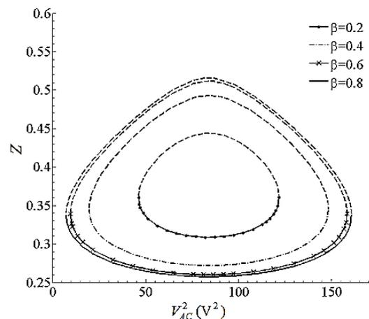
Fig. 12. Averaged position of vibration versus square of AC voltage amplitude for  $\Omega=272\text{ kHz}$  and relative crack depth  $n=0.5$  and different relative crack locations  $\beta$
