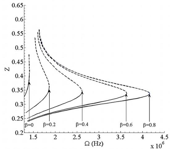
**Fig. 7. Averaged position of vibration versus excitation frequency for  $V_{DC}=5.7$  V,  $V_{AC}=9.88$  V and relative depth ratio  $n=0.5$  and different relative crack locations  $\beta$**
