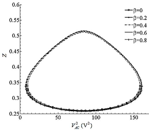
Fig. 8. Averaged position of vibration versus square of AC voltage amplitude for  $\Omega=272\text{ kHz}$  and relative crack depth  $n=0.1$  and different relative crack locations  $\beta$
