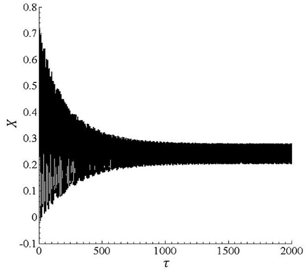
**Fig. 14. Time history of Eq. (18) for cracked micro-beam with relative crack depth  $n=0.3$  and relative crack location  $\beta=0.4$  for  $\alpha=0.1509$ ,  $\gamma=0.07$  and  $\Omega_{non}=3.1$**
