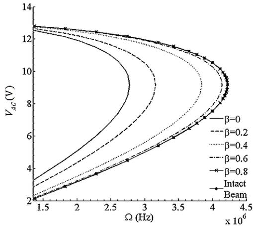
Fig. 16. Suppression zone of the pull-in instability versus  $V_{DC}^2 + V_{AC}^2 / 2 = 81.33$  and relative depth ratio  $n = 0.2$  and different relative crack locations  $\beta$
