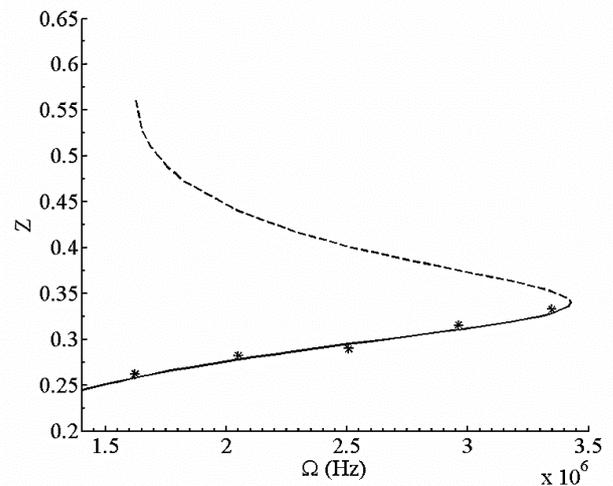
Fig. 20. Averaged position of vibration versus excitation frequency for  $V_{DC} = 5.7$  V,  $V_{AC} = 9.88$  V,  $n = 0.3$  and  $\beta = 0.4$ : using direct partition of motion method (-) and Runge–Kutta method (\*)
