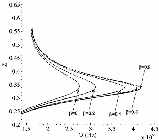
**Fig. 4. Averaged position of vibration versus excitation frequency for  $V_{DC}=5.7$  V,  $V_{AC}=9.88$  V and relative depth ratio  $n=0.2$  and different relative crack locations  $\beta$**
