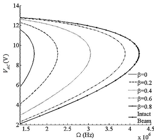
Fig. 18. Suppression zone of the pull-in instability versus  $V_{DC}^2 + V_{AC}^2 / 2 = 81.33$  and relative depth ratio  $n = 0.4$  and different relative crack locations  $\beta$
