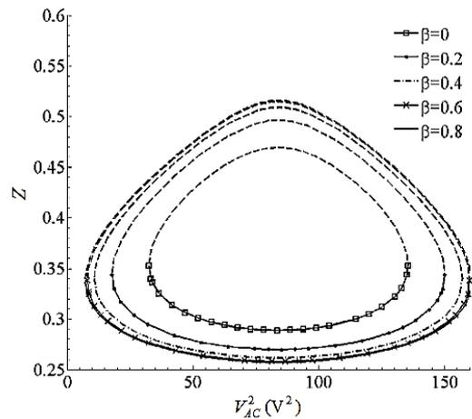
Fig. 11. Averaged position of vibration versus square of AC voltage amplitude for  $\Omega=272\text{ kHz}$  and relative crack depth  $n=0.4$  and different relative crack locations  $\beta$
