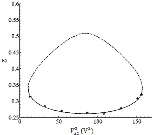
**Fig. 21. Averaged position of vibration versus square of AC voltage amplitude for  $\Omega=272$  kHz,  $n=0.3$  and  $\beta=0.4$ : using direct partition of motion method (-) and Runge-Kutta method (\*)**
