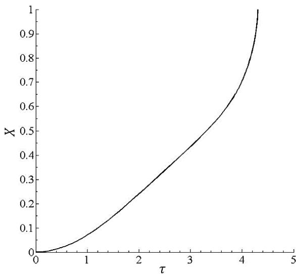
**Fig. 13. Time history of Eq. (3) for cracked micro-beam with relative crack depth  $n=0.3$  and relative crack location  $\beta=0.4$  for  $\alpha=0.1509$ ,  $\lambda=\gamma=0$**
