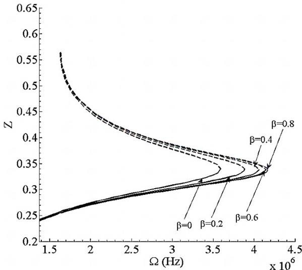
**Fig. 3. Averaged position of vibration versus excitation frequency for  $V_{DC}=5.7$  V,  $V_{AC}=9.88$  V and relative depth ratio  $n=0.1$  and different relative crack locations  $\beta$**
