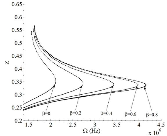
**Fig. 5. Averaged position of vibration versus excitation frequency for  $V_{DC}=5.7$  V,  $V_{AC}=9.88$  V and relative depth ratio  $n=0.3$  and different relative crack locations  $\beta$**
