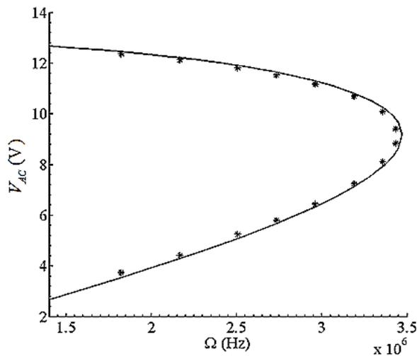
**Fig. 22. Suppression zone of the pull-in instability versus  $V_{DC}^2 + V_{AC}^2/2=81.33$  and for  $n=0.3$  and  $\beta=0.4$ : using direct partition of motion method (-) and Runge-Kutta method (\*)**
