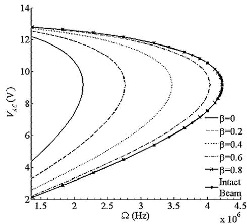
Fig. 17. Suppression zone of the pull-in instability versus  $V_{DC}^2 + V_{AC}^2 / 2 = 81.33$  and relative depth ratio  $n = 0.3$  and different relative crack locations  $\beta$
