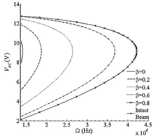
Fig. 19. Suppression zone of the pull-in instability versus  $V_{DC}^2 + V_{AC}^2 / 2 = 81.33$  and relative depth ratio  $n = 0.5$  and different relative crack locations  $\beta$
