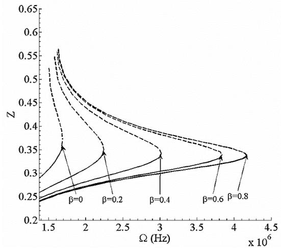
**Fig. 6. Averaged position of vibration versus excitation frequency for  $V_{DC}=5.7$  V,  $V_{AC}=9.88$  V and relative depth ratio  $n=0.4$  and different relative crack locations  $\beta$**
