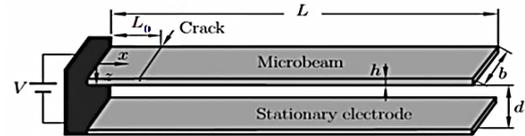
Fig. 1. A schematic view of electrically actuated cracked cantilever micro-beam
