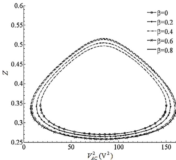
Fig. 9. Averaged position of vibration versus square of AC voltage amplitude for  $\Omega=272\text{ kHz}$  and relative crack depth  $n=0.2$  and different relative crack locations  $\beta$
