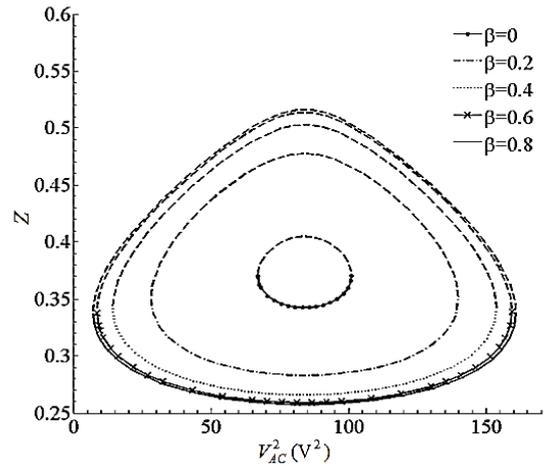
Fig. 10. Averaged position of vibration versus square of AC voltage amplitude for  $\Omega=272\text{ kHz}$  and relative crack depth  $n=0.3$  and different relative crack locations  $\beta$
