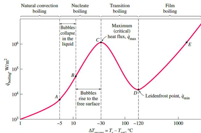
Fig. 1. Pool boiling curve for water at 1 atm [3]
