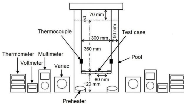
**Fig. 3. Schematic of the equipment and pool dimensions**
