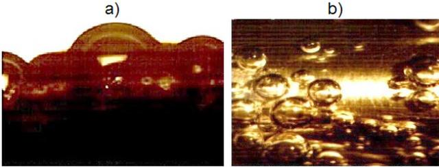
**Fig. 7. Photographs from boiling process, (a) Side view of bubble formation, (b) Top view of bubble departure**
