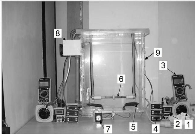
**Fig. 2. Experimental setup, (1) Variac, (2) Voltmeter, (3) Multimeter, (4) Thermometer, (5) Preheater, (6) Test case, (7) Switch, (8) Pump, (9) Pool**
