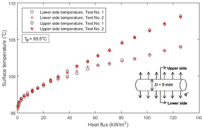
**Fig. 8. Repeatability of experimental measurements**
