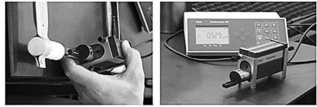
**Fig. 6. Surface roughness measuring device, Mahr M2 Perthometer, and typical output**
