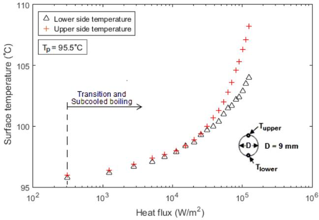
**Fig. 12. Variation of surface temperature with respect to the heat flux in saturated boiling**
