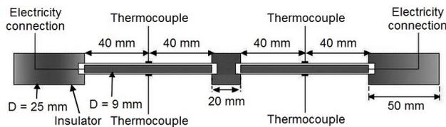
**Fig. 5. Dimensions of the test case and location of the thermocouples**
