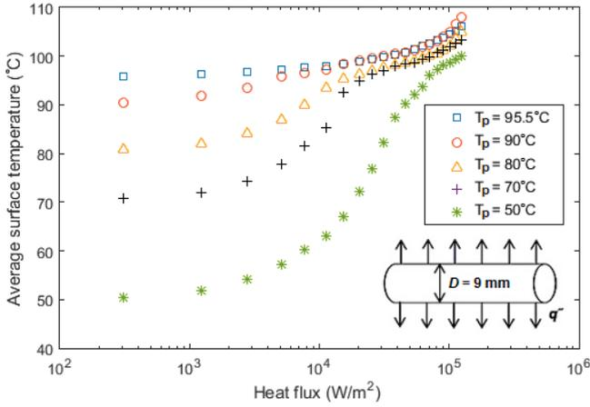
**Fig. 15. Effect of subcooling degree on average surface temperature**
