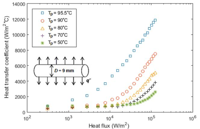
**Fig. 14. Effect of subcooling degree on heat transfer coefficient**
