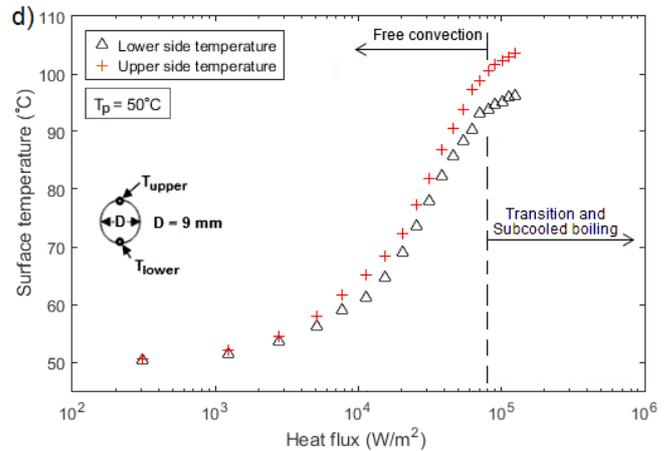
**Fig. 13. Variation of surface temperature with respect to the heat flux in subcooled boiling**
