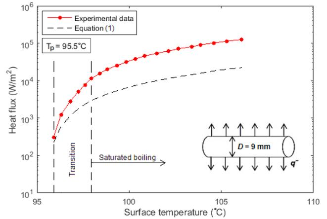
**Fig. 9. Comparison between saturated boiling and natural convection**
