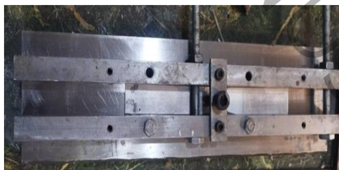
Fig. 1. Adhesive curing fixture designed for specimen placement and alignment control.
