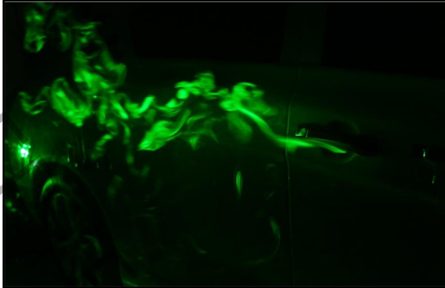
Fig. 6 Visualization of the flow passing through car handles
