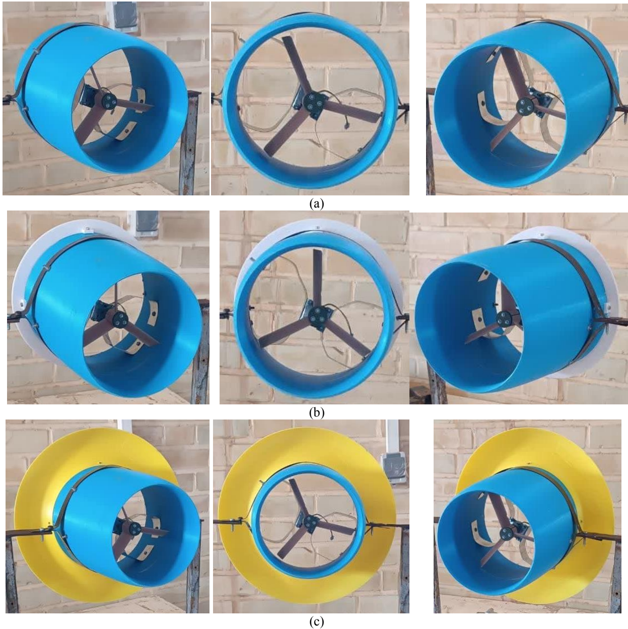
Fig. 7. a) Shroud + turbine, b) Shroud + vertical flange + turbine, c) Shroud + curved flange + turbine.
