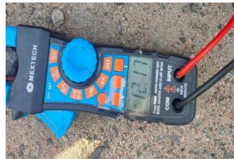
Voltage rating of solar panel
