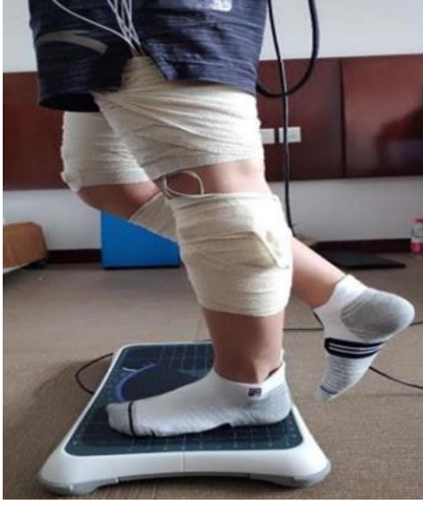
Fig. 1. Test procedure for standing on the left foot.
