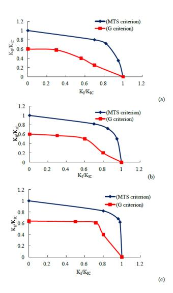
Fig. 20. Comparison of fracture toughness determined using the two criteria: (a) pure epoxy, (b) 1.5 wt. % nanotubes nanocomposite, (c) 3 wt. % CNT nanocomposite (sinusoidal, randomly distributed).
