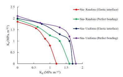
Fig. 14. Comparison between perfect bonding and elastic interface for nanocomposite reinforced with sinusoidal carbon nanotubes.
