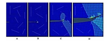
Fig. 7. Crack growth in nanocomposite reinforced with randomly distributed straight CNTs. (A) to (D) show crack growth path in the nanocomposite.
