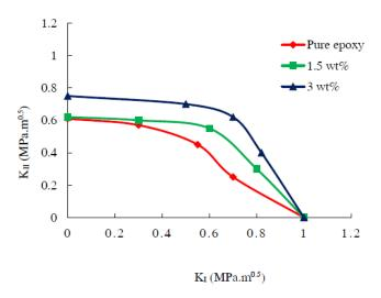
Fig. 19. KI-KIc curves for the nanocomposite reinforced with randomly distributed sinusoidal CNTs (G).
