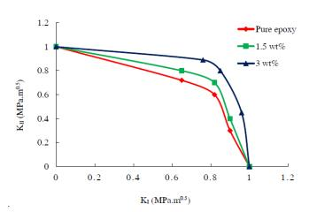
Fig. 18. KI-KIc curves for the nanocomposite reinforced with randomly distributed sinusoidal CNTs (MTS).
