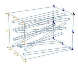
Fig. 2. The FEA model of the RVE under mixed mode loading (randomly distributed).
