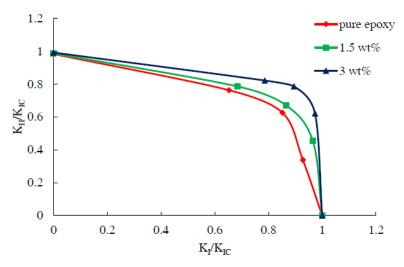
Fig. 16. KI-KIc curves for the nanocomposite reinforced with randomly distributed straight CNTs.
