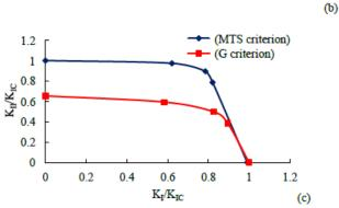
Fig. 17. Comparison of fracture toughness determined using the two criteria: (a) pure epoxy, (b) 1.5 wt. % CNT nanocomposite, (c) 3 wt. % CNT nanocomposite (randomly distributed).
