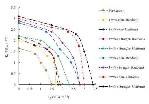
Fig. 10. Comparison of nanocomposites reinforced with straight and sinusoidal carbon nanotubes, randomly and uniformly distribution.
