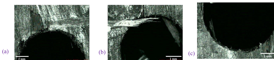
Fig. 10. Illustration of the drilled holes by a) HSS, b) HSS-5% Co, c) HSS-8% Co.
