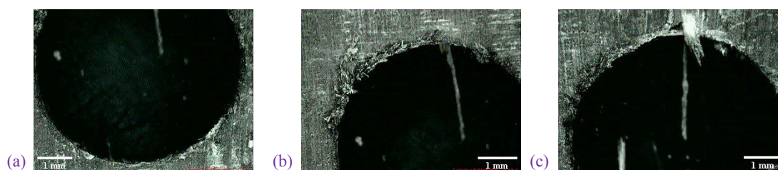
Fig. 11. Illustration of the drilled holes in the feed rate of a) 0.08, b) 0.15, c) 0.25 mm/rev.
