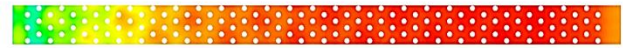
Fig.20: Cooling efficiency distribution contour on a flat plate with a blowing ratio of 1.5
