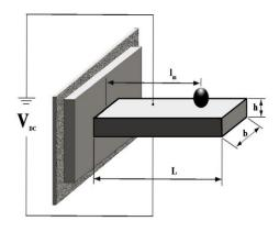
Fig. 1. Schema of an isotropic flexielectric micro-beam
