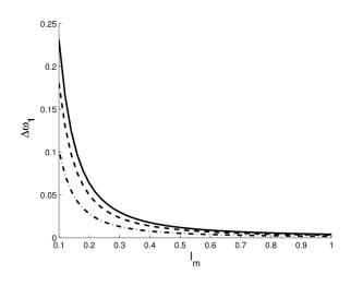
Fig. 9. The first frequency shift of FCMS for different effect of the material length scale factor with respect to the beam thickness ratio: l/h = 0.0, solid-lines, l/h = 0.2L, dashed-lines, and l/h = 0.5, dotted-dashed-lines
