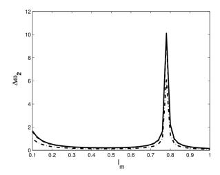
Fig. 10. The second frequency shift of FCMS for the different effect of the material length scale factor with respect to the beam thickness ratio: l/h = 0.0, solid-lines, l/h = 0.2L, dashed-lines, and l/h = 0.5, dotted-dashed-lines
