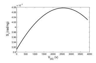
Fig. 12. The sensitivity in terms of applied DC voltage for 1/h = 0
