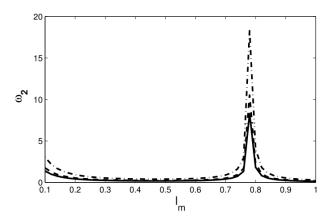
Fig. 4. The second frequency of FCMS for different the effect of the length scale parameter to the beam thickness ratio, i.e. l/h: l/h = 0.0, solid-lines, l/h = 0.2, dashed-lines, and l/h = 0.5, dotted-dashed-lines
