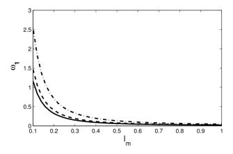
Fig. 3. The first frequency of FCMS for different the effect of the length scale parameter to the beam thickness ratio, i.e. l/h: l/h = 0.0, solid-lines, l/h = 0.2, dashed-lines, and l/h = 0.5, dotted-dashed-lines.
