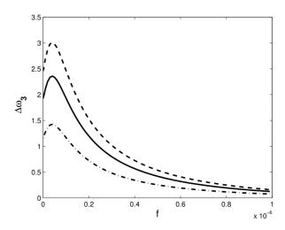
Fig. 8. The third frequency shift of FCMS for different position of the added mass: lm = 0.2L, solid-lines, lm = 0.6L, dashed-lines, and lm = L, dotted-dashed-lines
