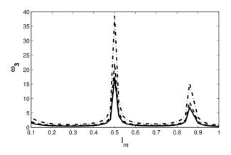
Fig. 5. The third frequency of FCMS for different the effect of the length scale parameter to the beam thickness ratio, i.e. l/h: l/h = 0.0, solid-lines, l/h = 0.2, dashed-lines, and l/h = 0.5, dotted-dashed-lines
