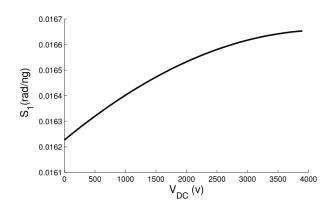
Fig. 15. The sensitivity in terms of applied DC voltage for the position of the added mass lm = 0.2L
