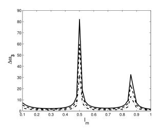
Fig. 11. The third frequency shift of FCMS for different effect of the material length scale factor with respect to the beam thickness ratio: l/h = 0.0, solid-lines, l/h = 0.2L, dashed-lines, and l/h = 0.5, dotted-dashed-lines
