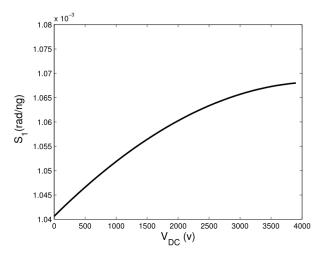
Fig. 14. The sensitivity in terms of applied DC voltage for position of the added mass lm = 1
