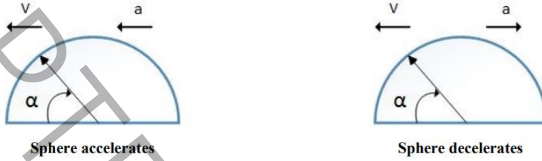
Fig. 1. Domain geometry and boundary conditions ( \alpha denotes the clockwise angle from the sphere leading edge.)
