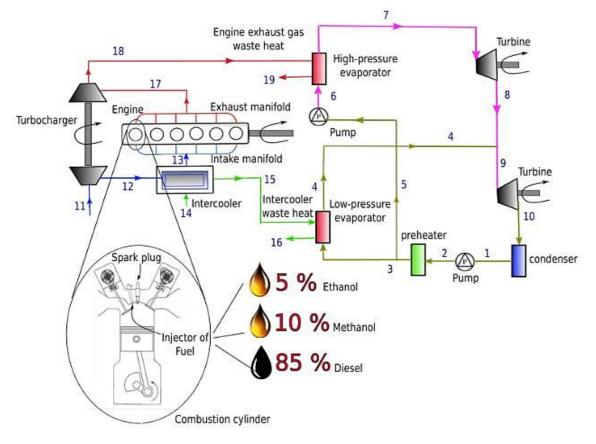
Fig. 1. The Dual-Pressure Organic Rankine Cycle (DPORC) utilizing the exhaust and coolant waste heat of the turbocharged diesel engine worked with ethanol/methanol mixtures
