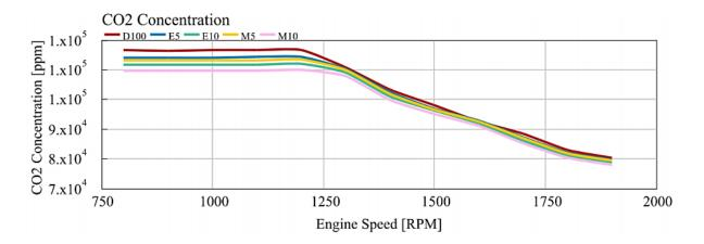
Fig. 7. CO2 emission for different fuels
