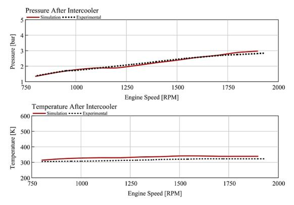
Fig. 3. Comparison of reported results with those of the simulation for pressure and temperature after intercooler.
