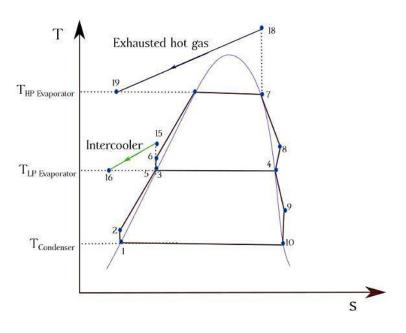
Fig. 2. T-S diagram of DPORC
