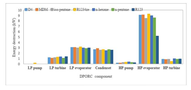
Fig. 15. Comparison of exergy destruction for seven working fluids for DPORC system by adding of D100 to Diesel.
