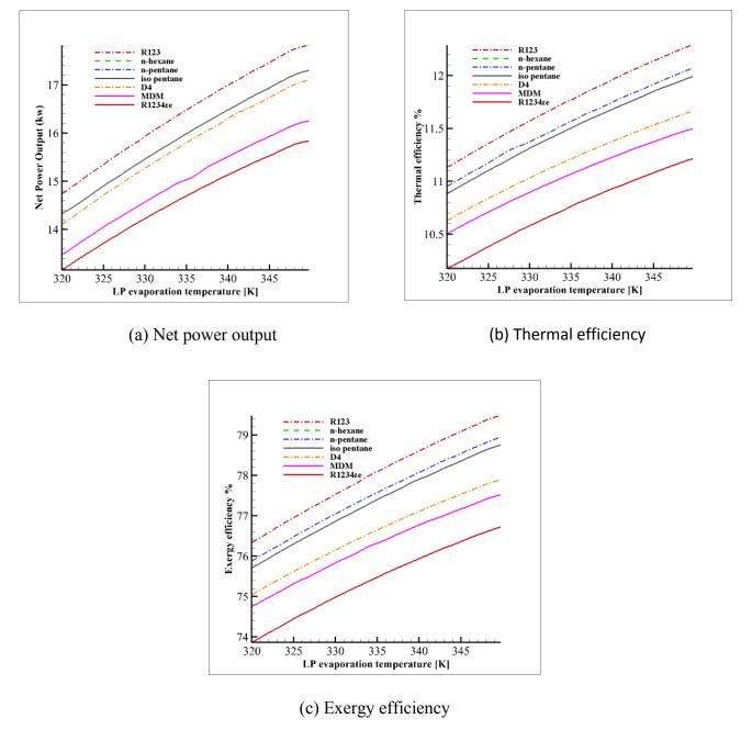
Fig. 11. Performance of the proposed system under the influence of LP evaporation temperature
