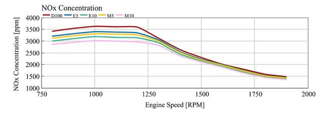
Fig. 8. NOx emission for different fuels
