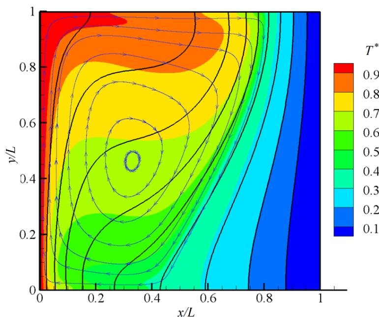
**Fig. 7. Temperature contour for the PCM and porous medium at  $Fo=0.002$  specified by the color spectrum and solid lines, respectively, in 9 levels along with streamlines in the liquid phase ( $Da=10^{-2}$ ).**
