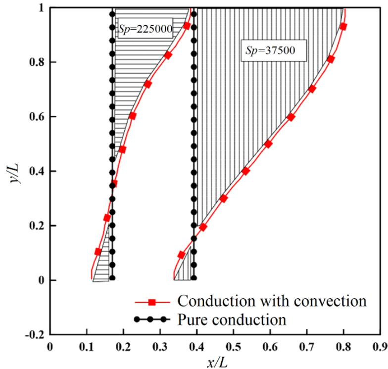
**Fig. 20. Position of melting front for pure conduction and natural convection at  $Fo=0.003$  and  $Da=10^{-2}$ .**
