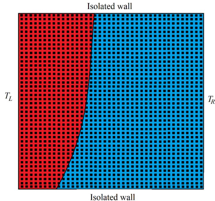
**Fig. 1. Schematic of melting problem inside a porous medium.**
