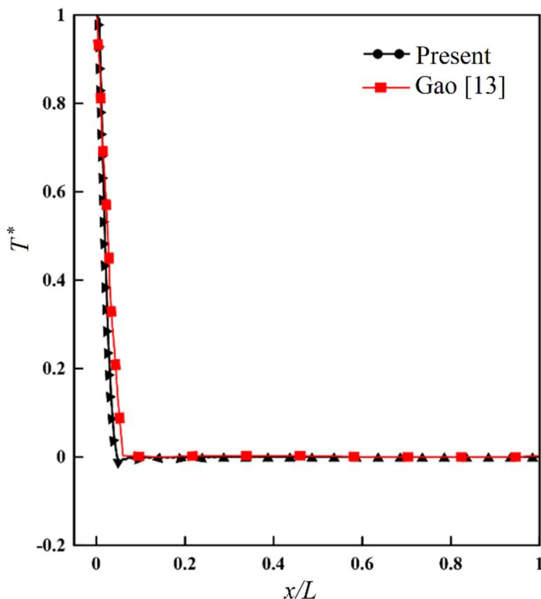
**Fig. 2. Temperature of the PCM on the line passing through the middle of the enclosure ( $y/L=0.5$ ) at  $Fo=0.002$  for the case of LTE.**
