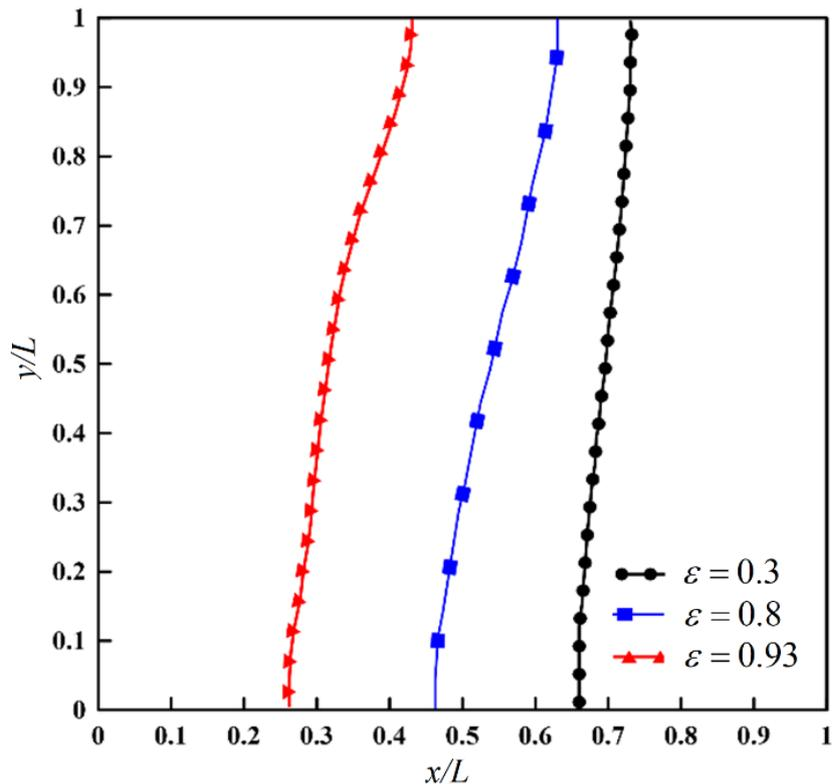
Fig.13. Position of the melting front at Fo=0.002 for three porosity ratios.
