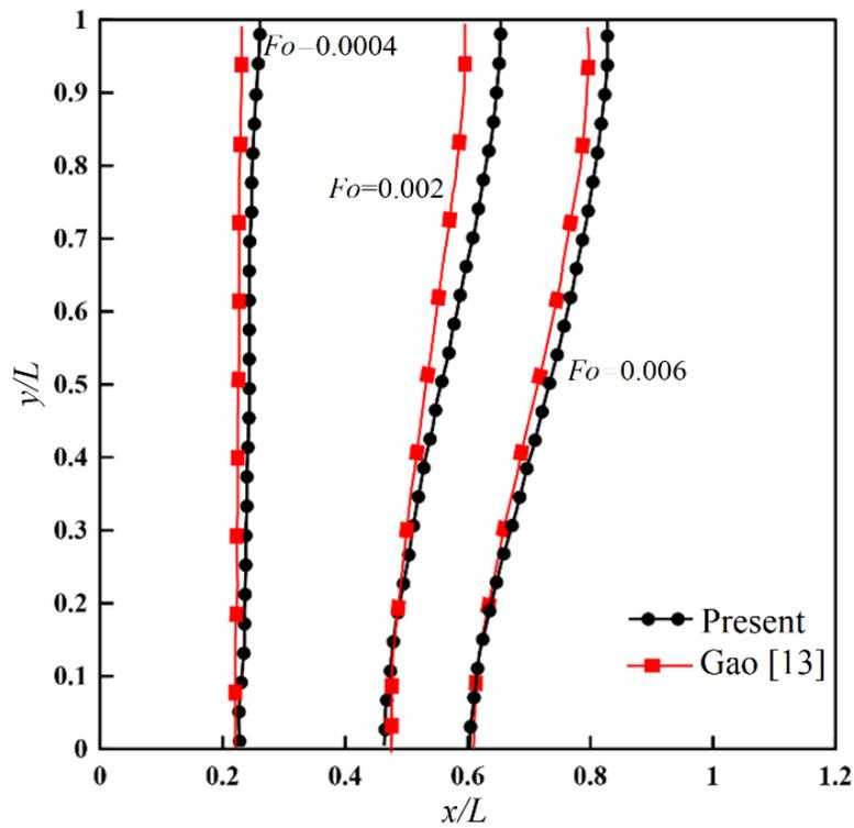
Fig. 5. Position of the melting front at  $Fo=0.0004$ ,  $Fo=0.002$ , and  $Fo=0.006$  for the case of LTNE.
