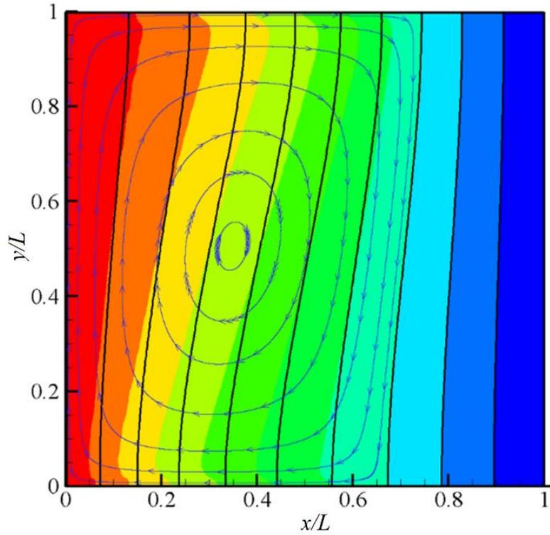
Fig. 11. Temperature contour for the PCM and porous medium at  $Fo=0.002$  specified by the color spectrum and solid lines, respectively, in 9 levels along with streamlines in the liquid phase ( $\varepsilon=0.3$ ).
