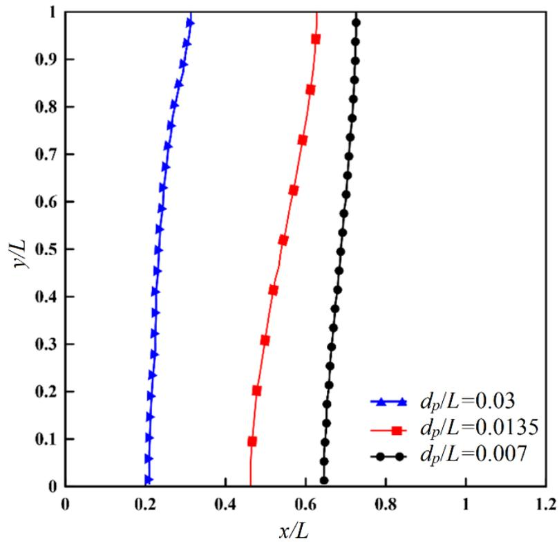
Fig. 15. Position of Melting front for different diameter to length ratios at Fo=0.002.
