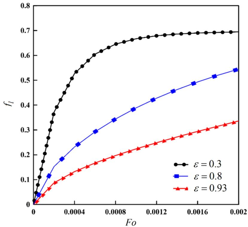
Fig. 12. Variation of the liquid fraction with respect to the time for three porosity ratios.
