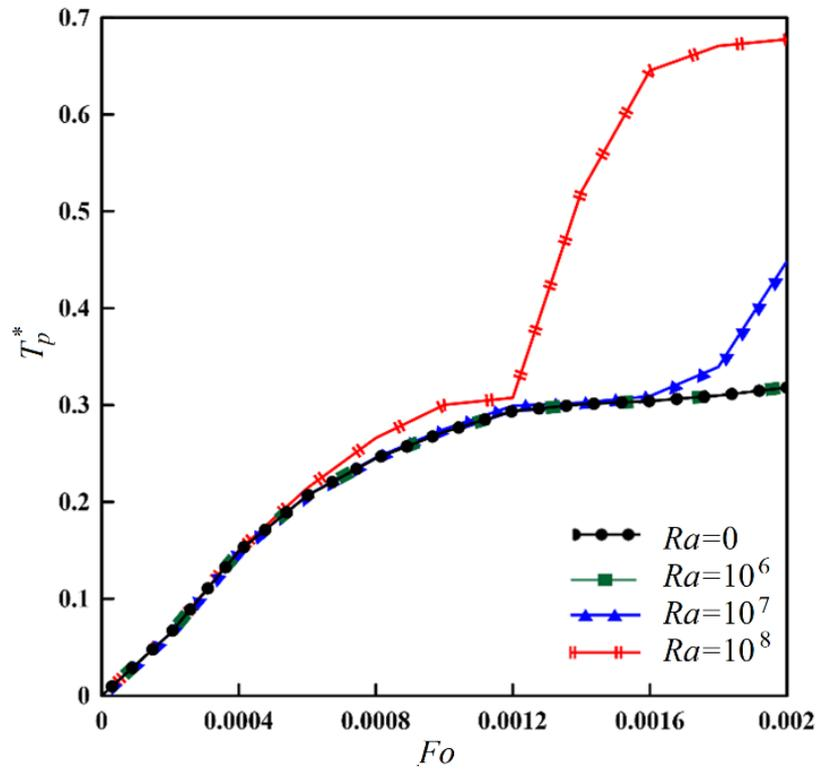
Fig. 10. Temperature of the node in the middle of the enclosure with time for different Rayleigh numbers.
