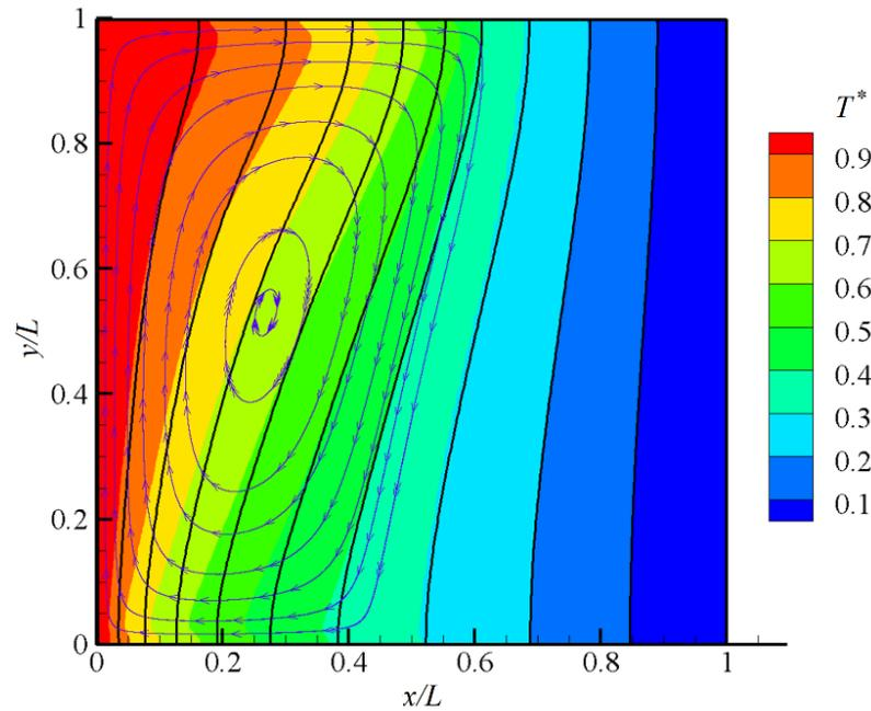
Fig. 4. Temperature contour for the porous medium specified by solid lines in 9 levels along with streamlines in the liquid phase. To compare the temperature of PCM and porous medium, the temperature of the PCM is given as a color spectrum.
