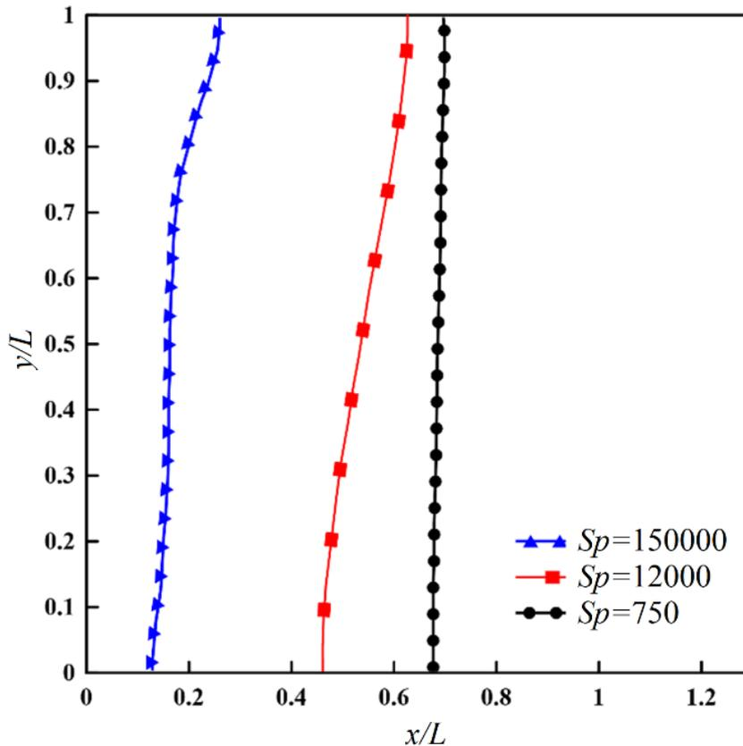
Fig. 17. The position of the melting front at  $Fo=0.002$  for different Sparrow numbers.
