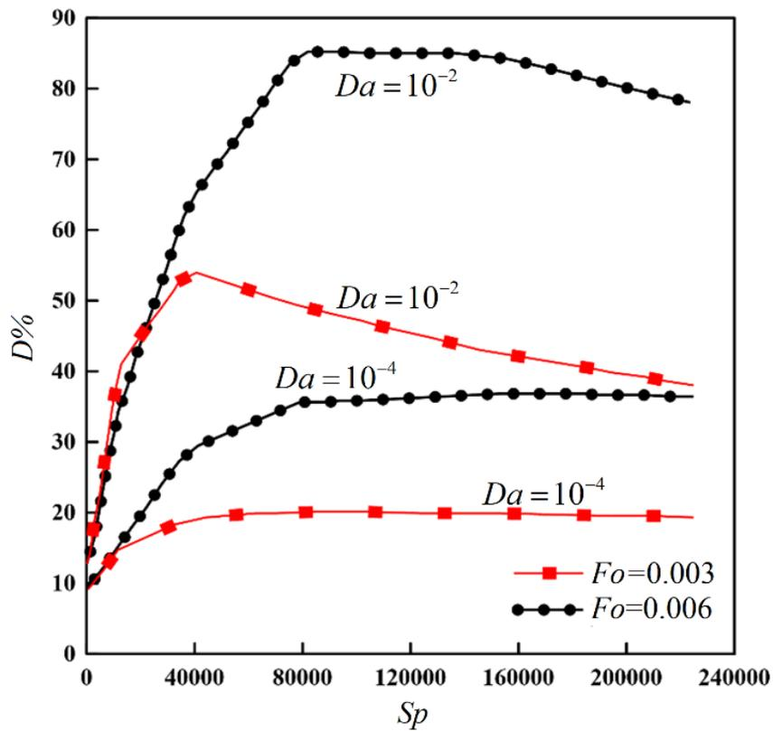
Fig. 19. Deviation of the liquid fraction compared to pure conduction under different Darcy and Sparrow numbers at Fo=0.003 and Fo=0.006.
