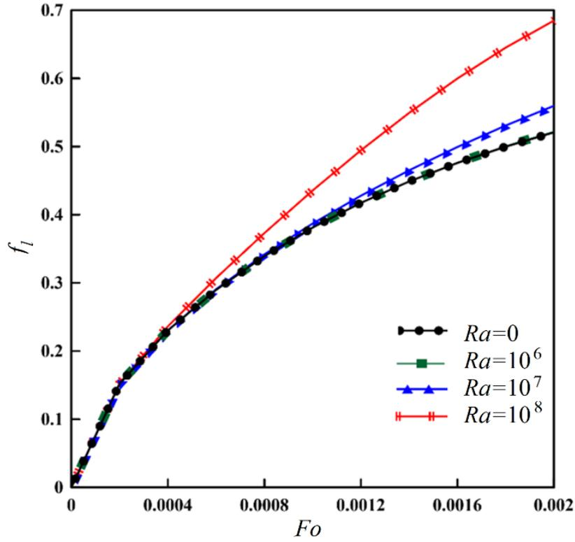
Fig. 8. Variation of the liquid fraction with respect to the dimensionless time at four Rayleigh numbers.
