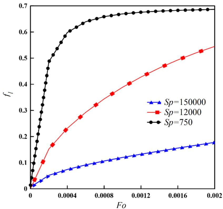
**Fig. 16. The liquid fraction variation with time for different Sparrow numbers.**
