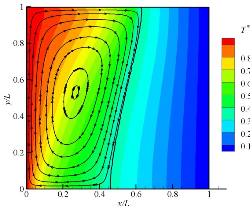
**Fig. 3. Temperature contour for the PCM at  $Fo=0.002$  specified by the color spectrum in 9 levels along with streamlines in the liquid phase (base condition).**
