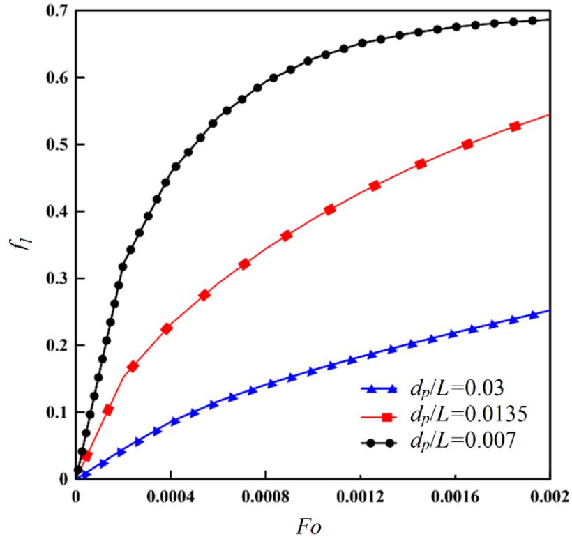
Fig. 14. Variation of liquid fraction for the different ratios of diameter to length.
