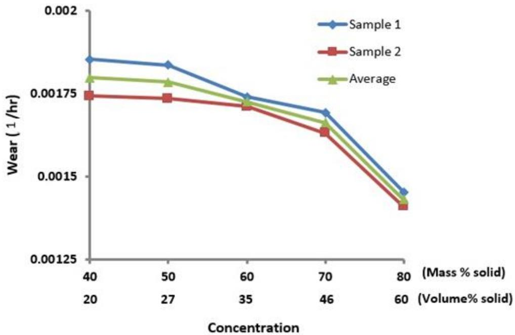
Fig. 8. Wear rate at a different slurry concentration in wet grinding ( $J_b=0.2$ ,  $\Phi_c=0.75$ ,  $U=1$ ).
