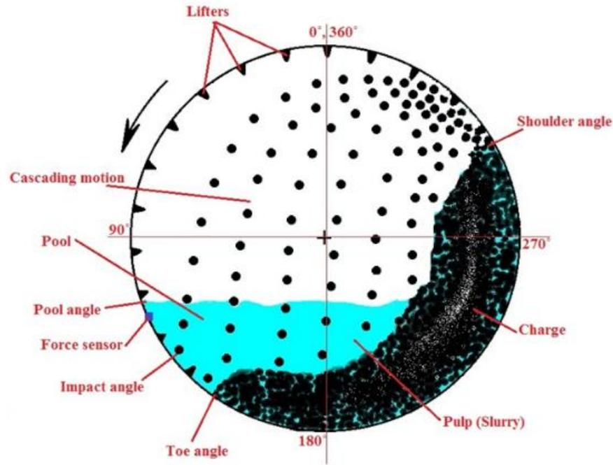
Fig. 1. Definition of the load behavior in a wet tumbling mill [5].
