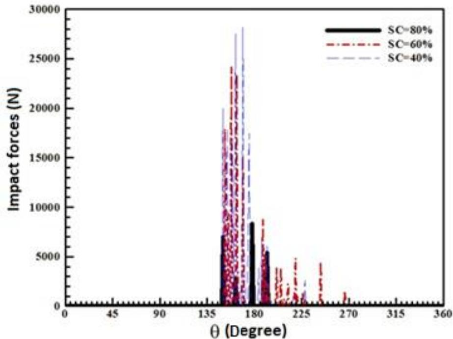
Fig. 9. Impact forces in one rotation of the mill at different concentrations ( $J_b=0.2$ ,  $\Phi_c=0.75$ ,  $U=1$ ).
