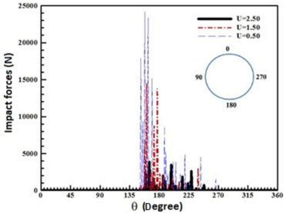
Fig. 7. Impact forces in one rotation of the mill at different slurry filling ( $J_b=0.2$ ,  $\Phi_c=0.75$ ,  $C=0.6$ ).
