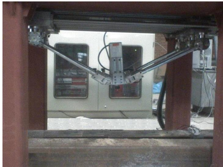
**Fig. 7. Six axes CNC Hexaglide machine**
