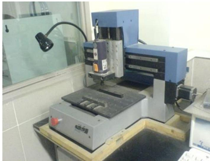
**Fig. 6. Three axes Kefa CNC machine**
