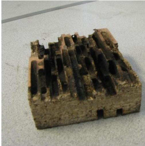
**Fig. 13. A workpiece with a ruined surface, the specified area is demanded to be smoothed**
