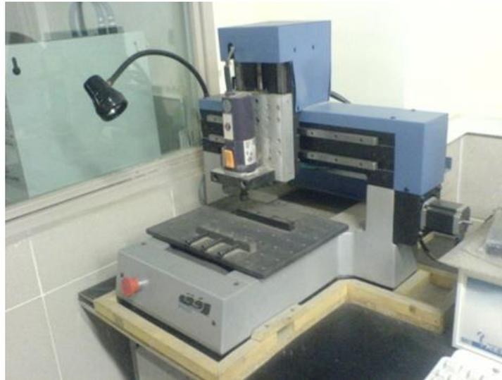
**Fig. 6. Three axes Kefa CNC machine**
