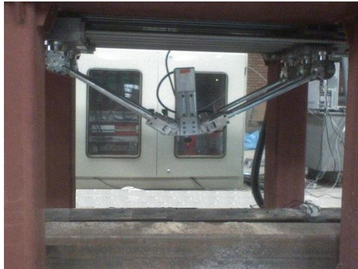
**Fig. 7. Six axes CNC Hexaglide machine**
