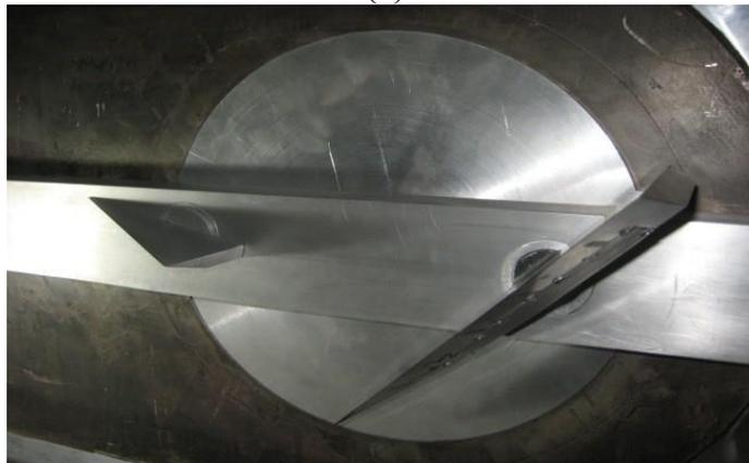
**Fig. 2. The model for high speed tests, (a) the schematic view, (b) the model installed on the sidewall**
