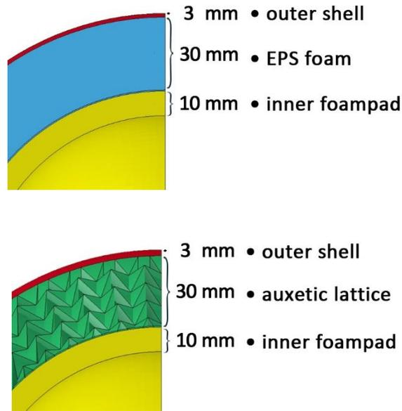
**Fig. 2.** Cross-sectional view of the modeled specimens. Top: Baseline helmet liner with EPS foam. Bottom: Helmet with innovative liner structure.
