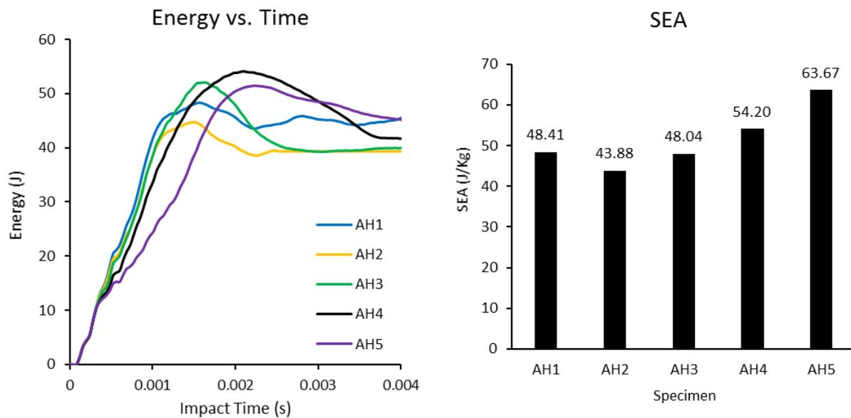
**Fig. 13. Comparison of energy absorption characteristics of modified helmets with different auxetic cell sizes: Left) Absorbed Energy, Right) Specific Energy Absorption.**
