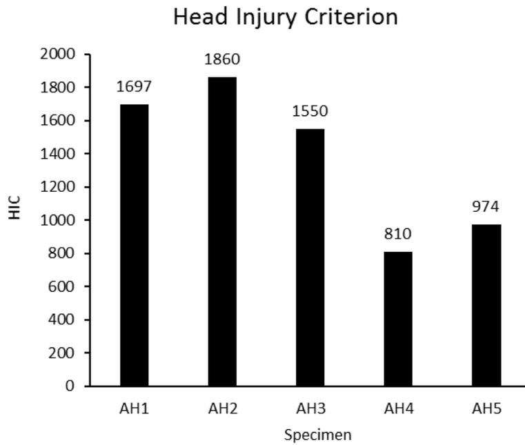
Fig. 12. HIC number of modified helmets with different auxetic cell sizes.
