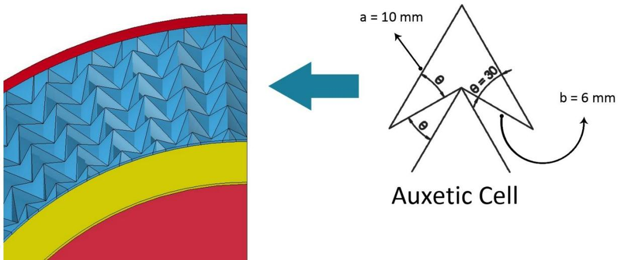
**Fig. 3.** Details of the auxetic structure employed in the proposed helmet liner.
