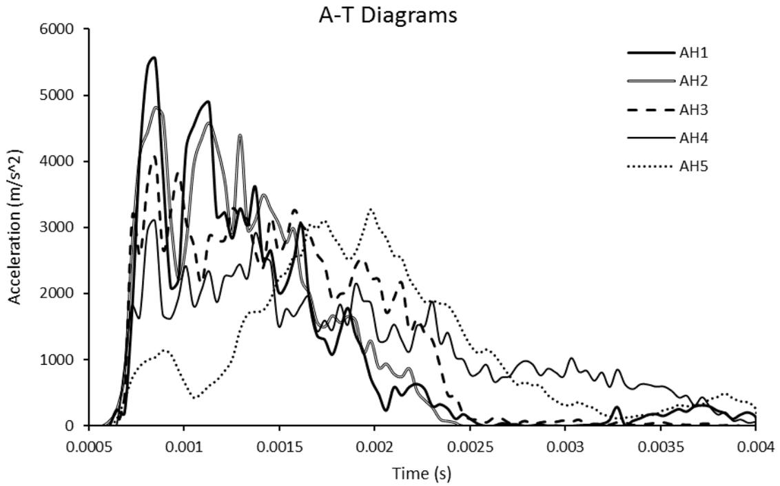
Fig. 11. Acceleration vs. time diagram of modified helmets with different auxetic cell sizes.
