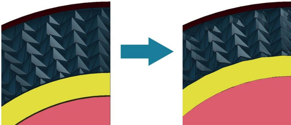
**Fig. 4.** deformation of the auxetic liner under blast loading.
