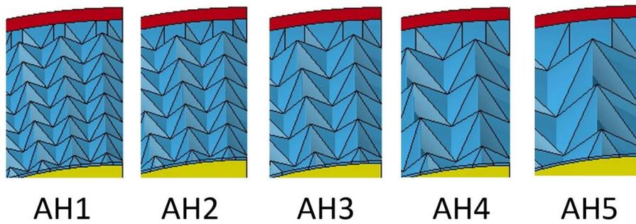
Fig. 9. Designs of the auxetic liner to achieve different densities.
