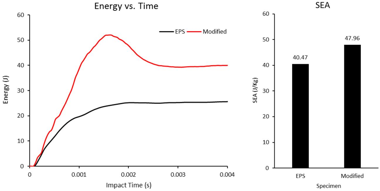
Fig. 8. Comparison of energy absorption characteristics of the modified helmet with baseline model under blast: Left) Absorbed Energy, Right) Specific Energy Absorption.
