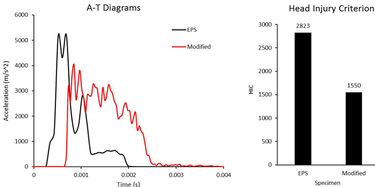
**Fig. 7. Comparison of the modified helmet with baseline model under blast: Left) Acceleration vs. time diagrams, Right) HIC numbers.**
