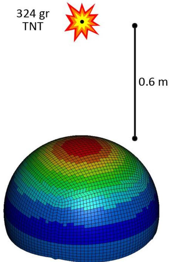
**Fig. 5.** Schematic of blast loading.
