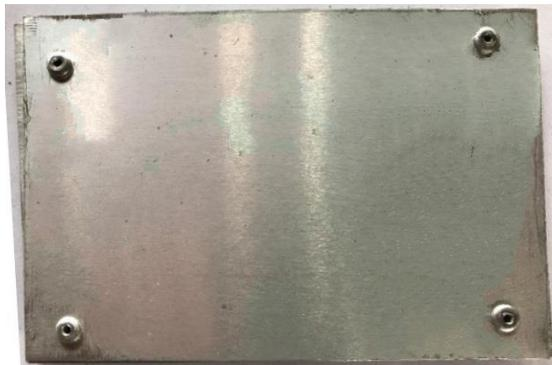
Prepared sample before FSP and after stacking and riveting
