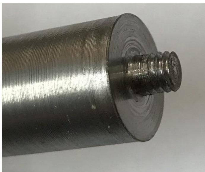
**Fig. 3. FSP tool used in this study.**
