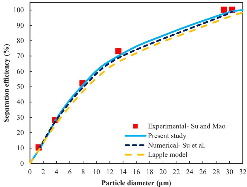
**Fig. 6. Comparison between the separation efficiency of the present study and experimental data [25], numerical results [9], and the Lapple model [45] at  $v=20 \text{ m/s}$**
