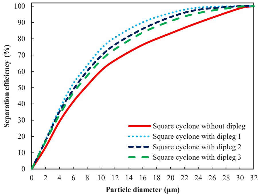
**Fig. 10. Comparison between the separation efficiency of a square cyclone with and without dipleg at  $v=20 \text{ m/s}$**
