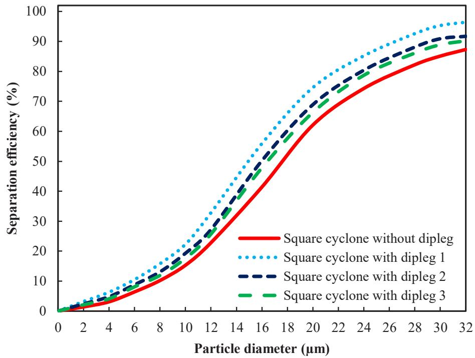
**Fig. 9. Comparison between the separation efficiency of a square cyclone with and without dipleg at  $v=12 \text{ m/s}$**
