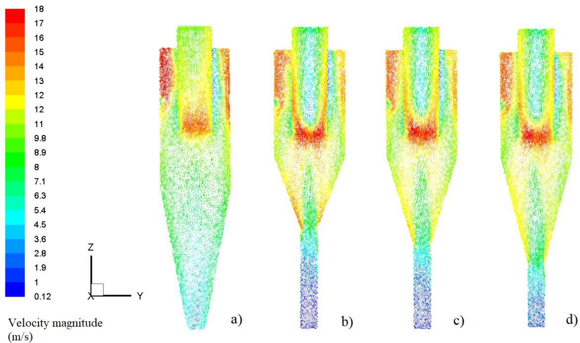
**Fig. 13. Velocity vector for square cyclone a) without dipleg b) with dipleg 1 c) with dipleg 2 d) with dipleg 3 at  $v=12$  m/s**
