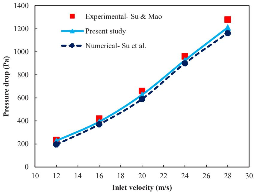
**Fig. 5. Comparison between the pressure drop of the present study and experimental data [25] and numerical results [9]**
