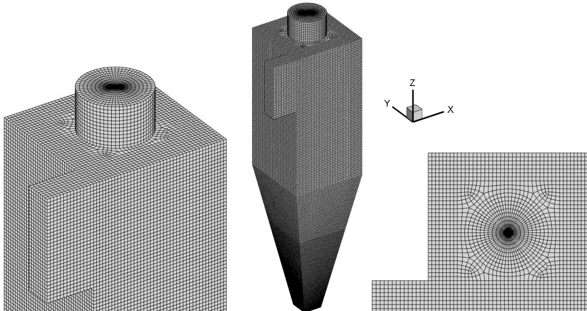
**Fig. 3. Computational grids for the base square cyclone**
