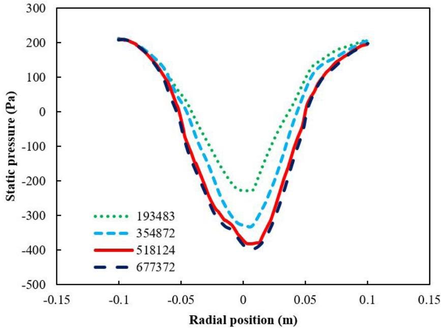
**Fig. 4. The radial profiles for the static pressure of square cyclone without dipleg at  $y=0.15$  m for different cell numbers at an inlet velocity of 20 m/s**
