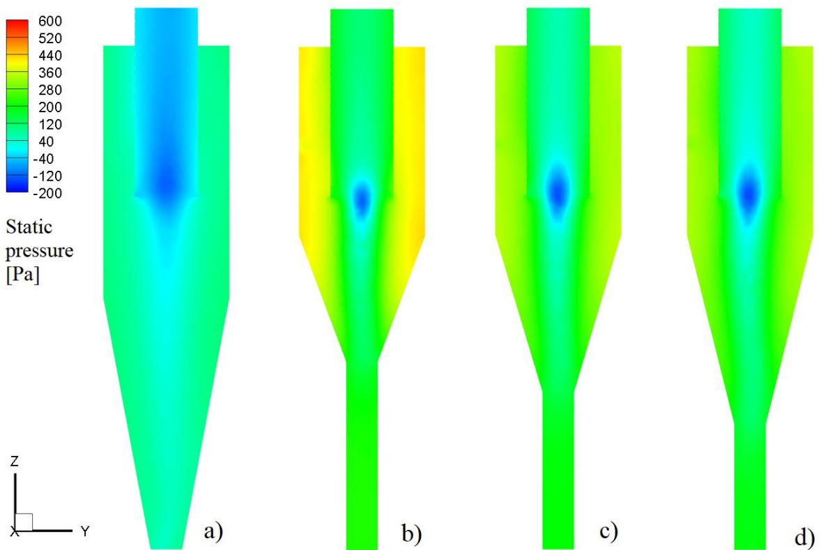
**Fig. 11. Contours of static pressure for square cyclone a) without dipleg b) with dipleg 1 c) with dipleg 2 d) with dipleg 3 at  $v=12 \text{ m/s}$**
