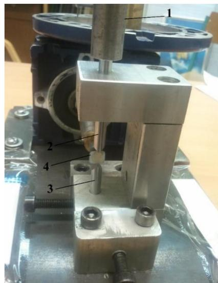
**Fig. 2. Loading fixture for performing force-frequency experiments**
