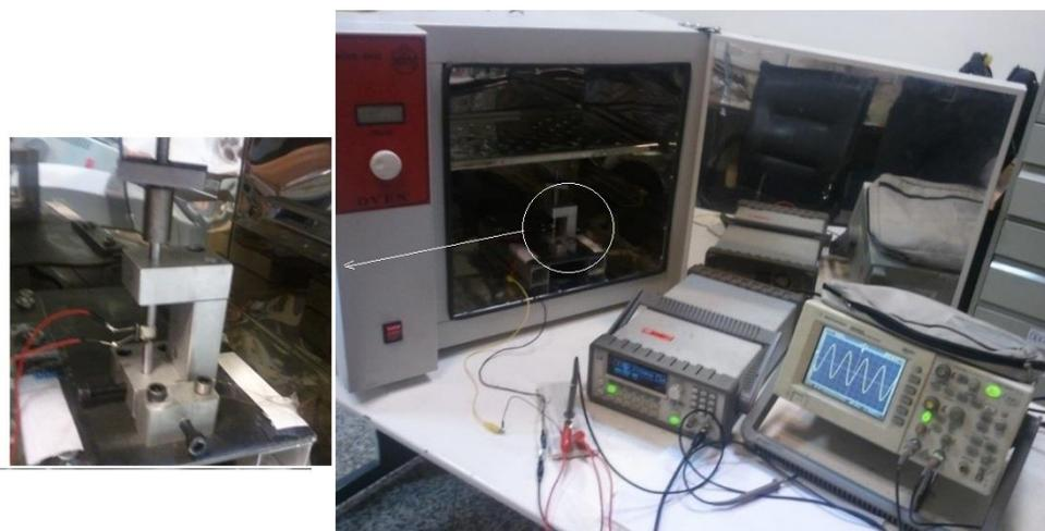
Fig. 3. Measuring the crystal frequency by a signal generator and an oscilloscope
