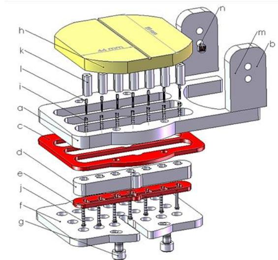
**Fig. 1. The fixture for temperature measurement [16]**
