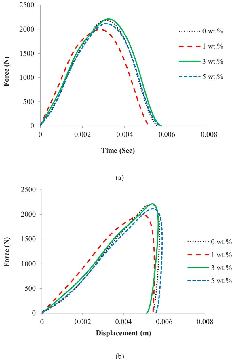
**Fig. 5. (a) Force-time history and (b) Force-displacement response of FMLs impacted at energy of 14.70 J**
