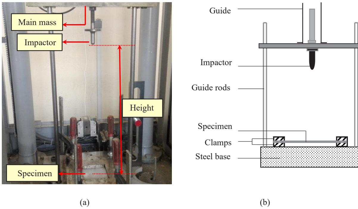
**Fig. 2. (a) Set-up for impact test (b) Schematic of the test set-up**
