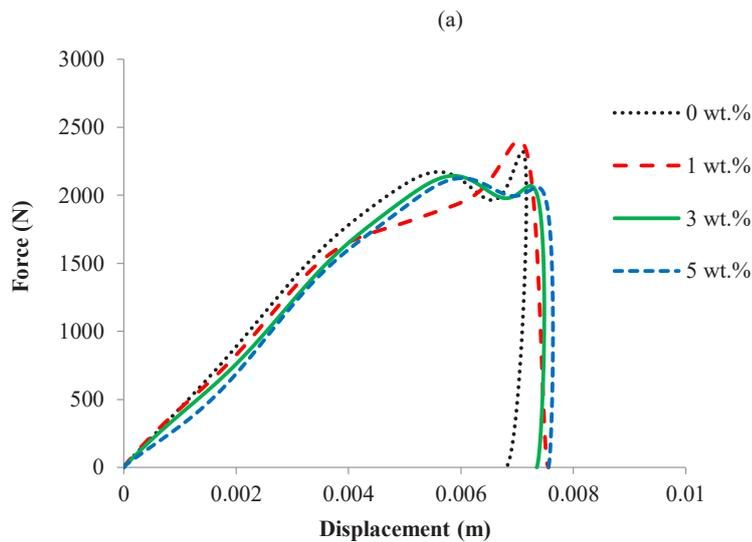
**Fig. 7. (a) Force-time history and (b) Force-displacement response of FMLs impacted at energy of 25.42 J**
