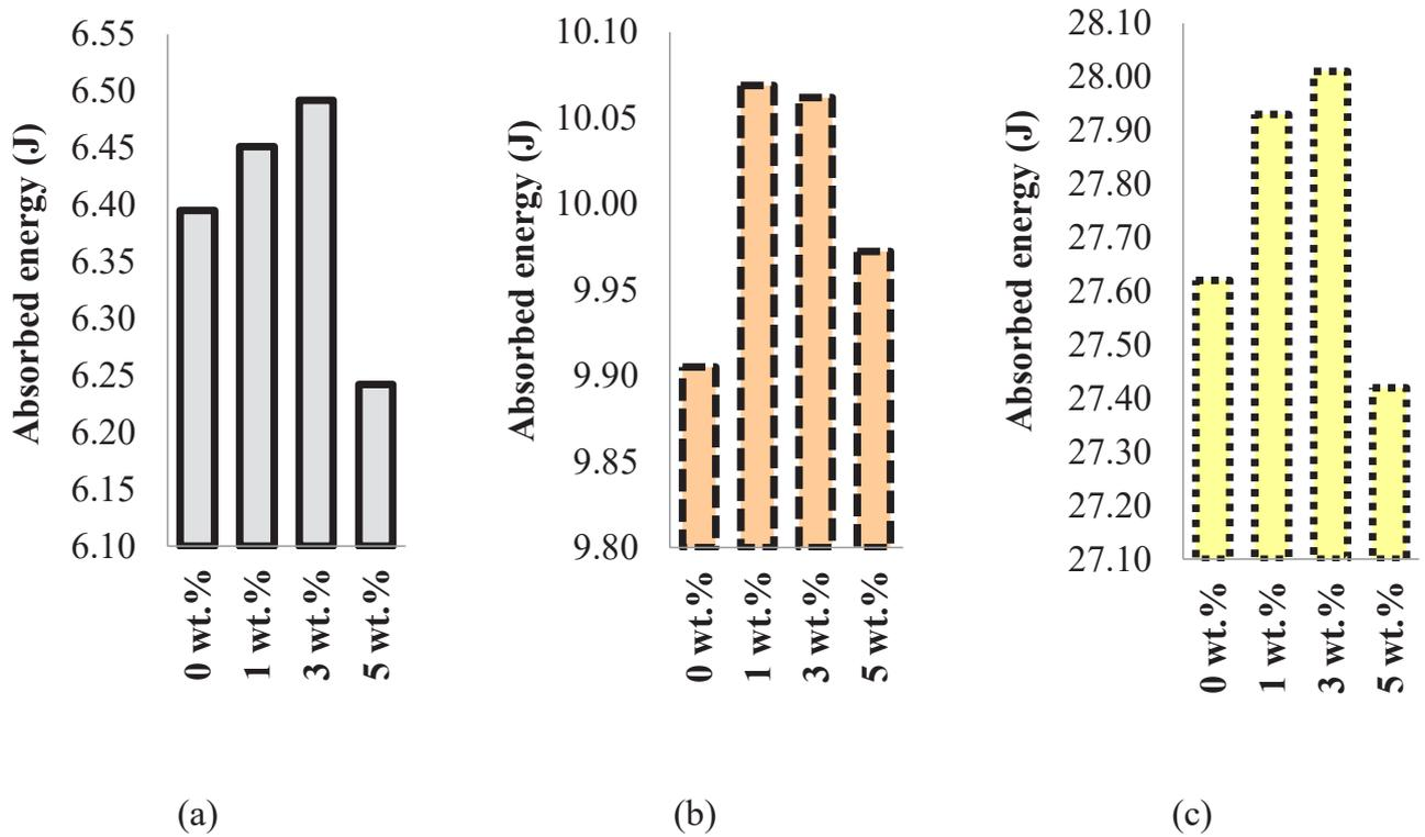
**Fig. 11. Comparison between the final absorbed energies considering various weight percentage of nanoclay, for impact energy levels of (a) 14.70, (b) 25.42 and (c) 27.99 J**
