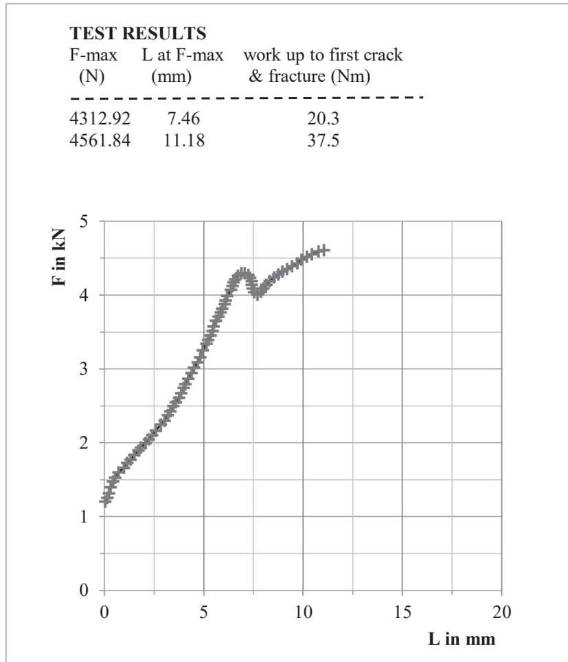
**Fig. 4. Force-displacement graph of quasi-static test**
