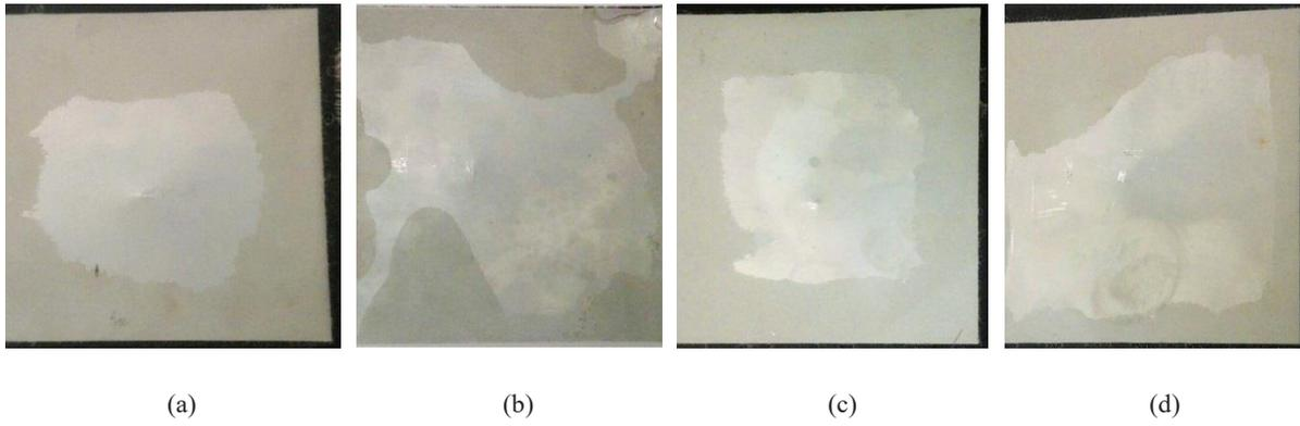
**Fig. 6. Damage patterns for the FMLs with (a) 0 wt.% (b) 1 wt.% (c) 3 wt.% (d) 5 wt.% of nanoclay struck with energy of 14.70J**
