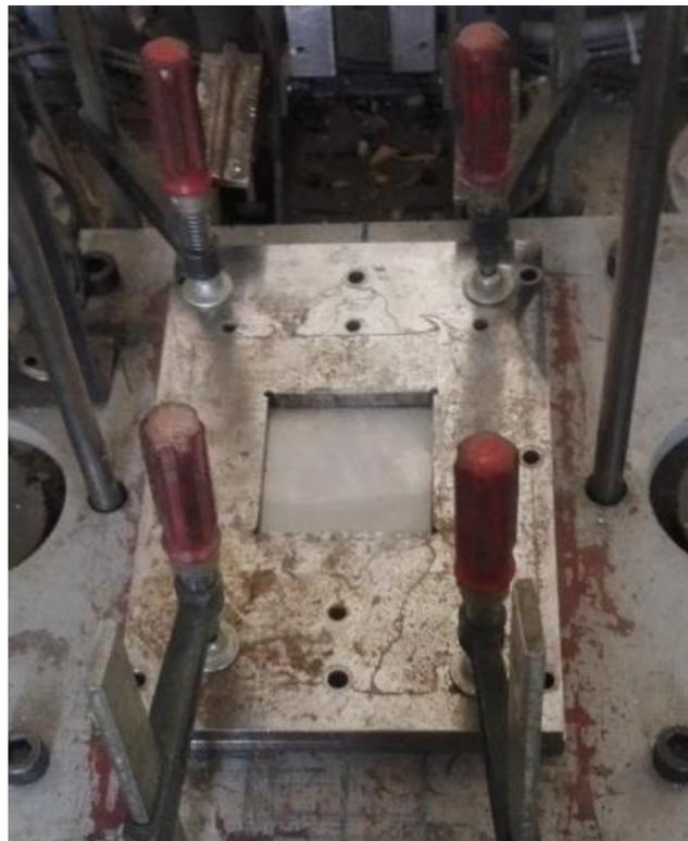
**Fig.3. Applying the fully clamped boundary conditions**
