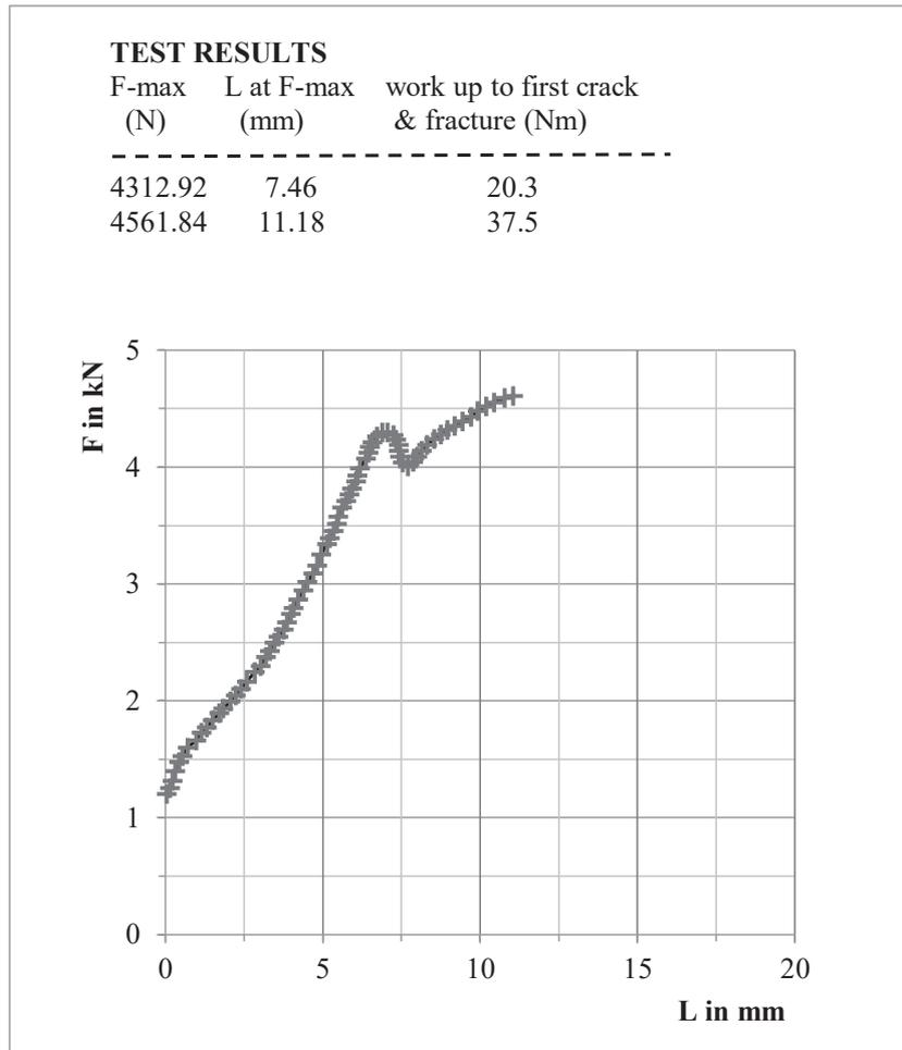
Fig. 4. Force-displacement graph of quasi-static test
