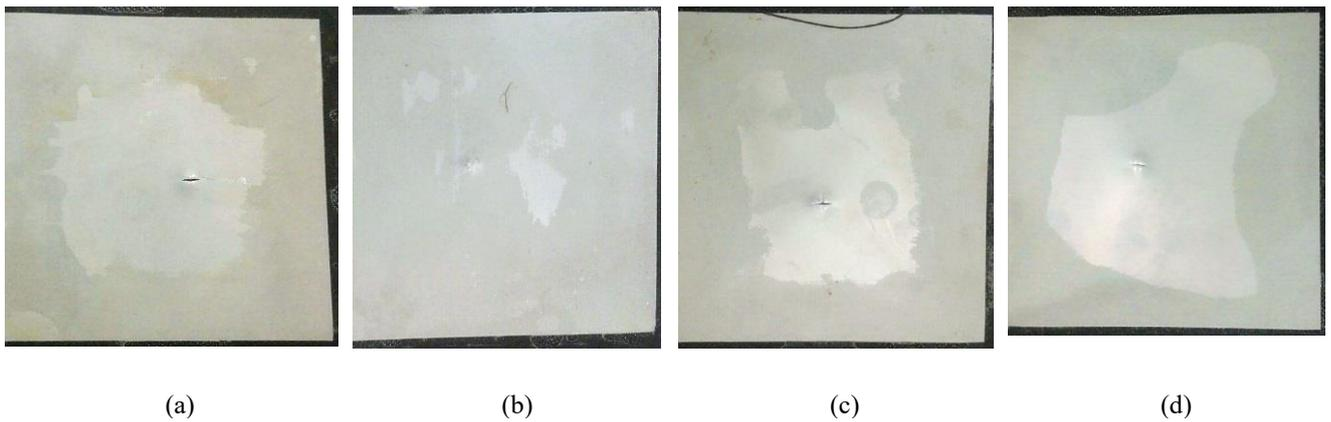
**Fig. 8. Damage patterns for the FMLs with (a) 0 wt.% (b) 1 wt.% (c) 3 wt.% (d) 5 wt.% of nanoclay struck with energy of 25.42J**
