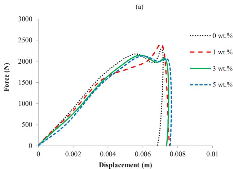
**Fig. 7. (a) Force-time history and (b) Force-displacement response of FMLs impacted at energy of 25.42 J**
