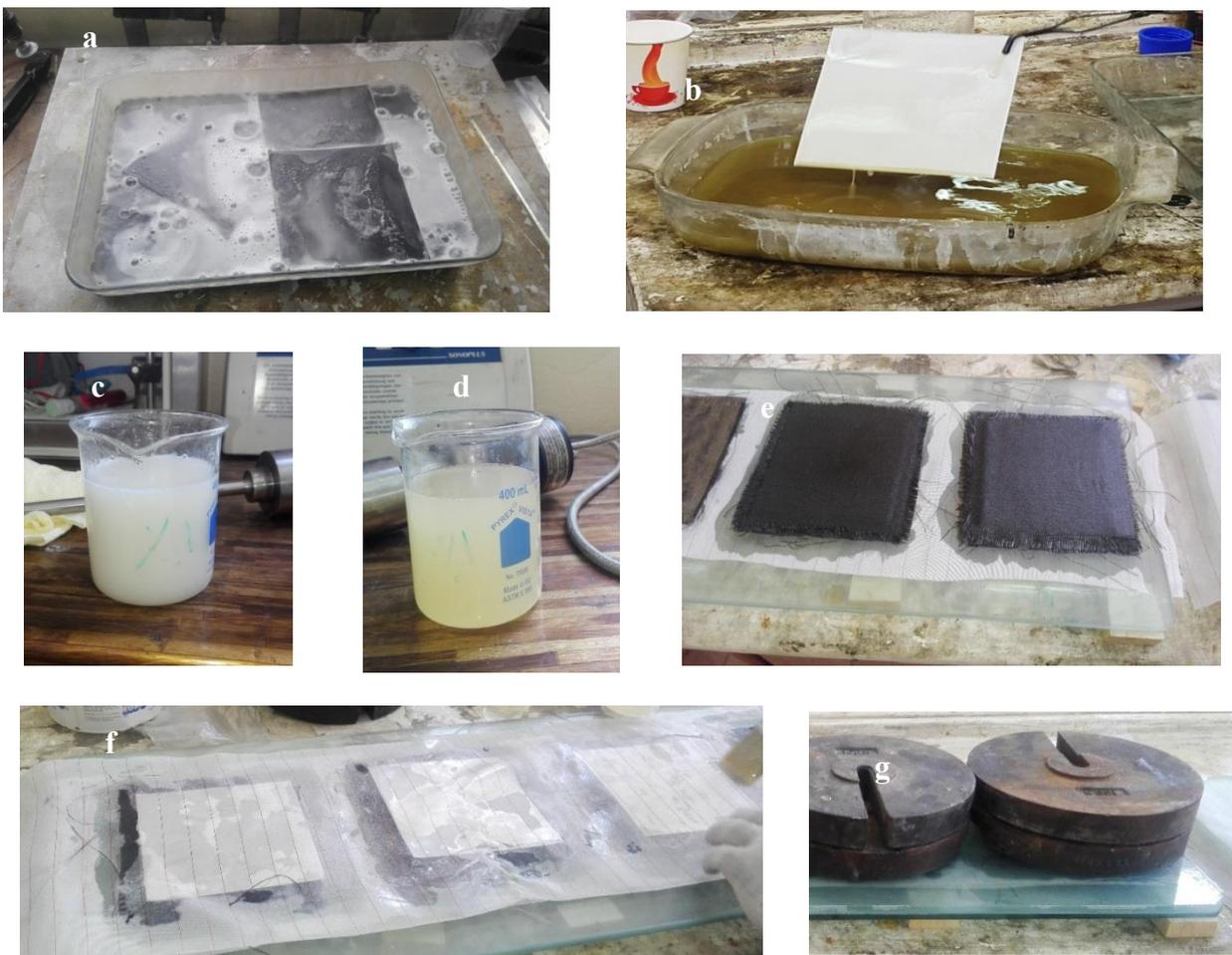
**Fig. 1. (a) The aluminum sheets immersed in alkaline solution. (b) The aluminum sheet after the etching process. (c) Resin-nanoclay mixture after mechanical mixing and (d) after ultrasonication. (e) Fabricating the specimens by placing the basalt fabrics between the prepared metal sheets using the hand lay-up technique. (f) Covering them with the Dacron fabric. (g) Applying the pressure for 24 hours.**
