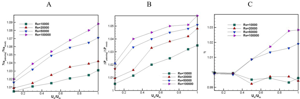
Fig. 10. A) The Nusselt number of pulsation flow to that of steady-state ratio variation, B) the pressure drop of pulsation flow to that of steady-flow variation, and C) thermal performance criteria with the ratio of the flow amplitude to that of the mean flow for various Reynolds number of water flow inside the helical-coil tube for  $d = 9$  mm and  $D = 112$  mm.
