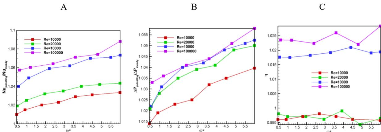
Fig. 12. A) Nusselt number of pulsation flow to that of steady-state variation, B) Pressure drop of pulsation flow to that of steady-state variation, C) Performance evaluation criteria, with nondimensional frequency for various Reynolds number of the nanofluid flow inside the helical-coil tube for  $d = 9$  mm and  $D = 112$  mm to the base fluid.
