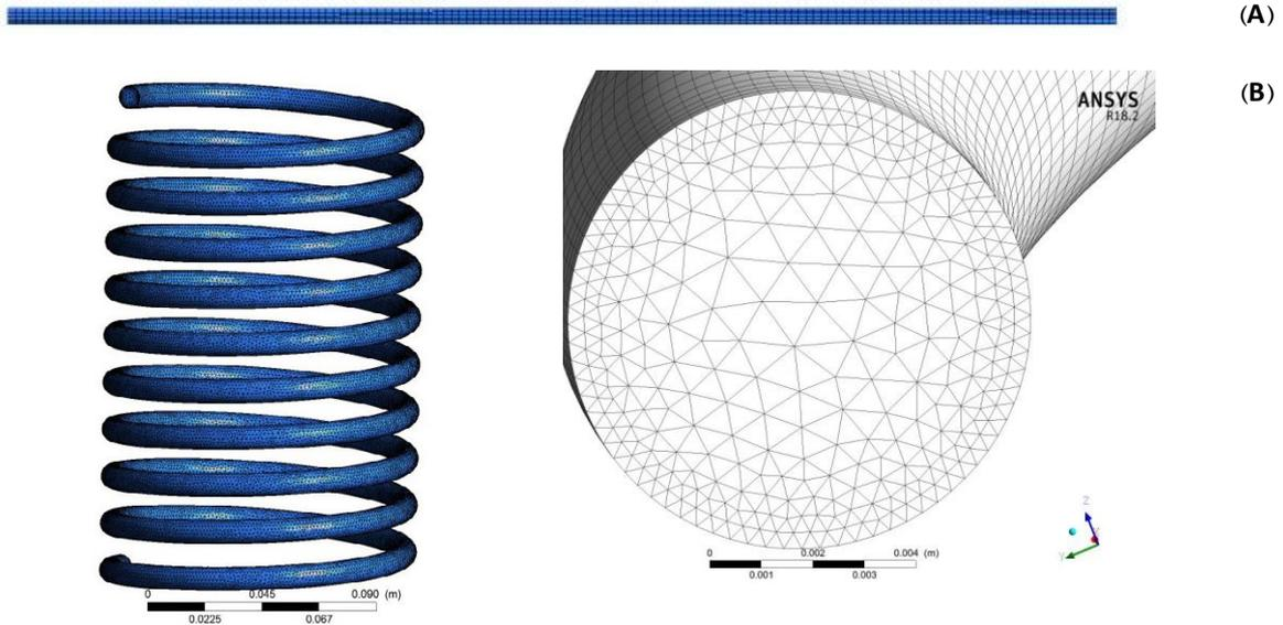
Fig. 2. The grid used in the grid independence test. A) Straight tube B) Helical-coil tube
