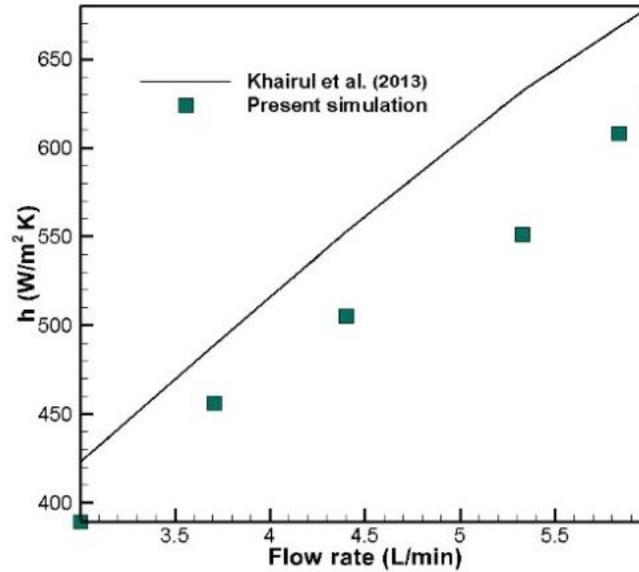
Fig. 5. Comparison between the present numerical simulation results for the heat transfer coefficient of coiled tube with the numerical results of Khairul et al. [30] for un-pulsation flow.
