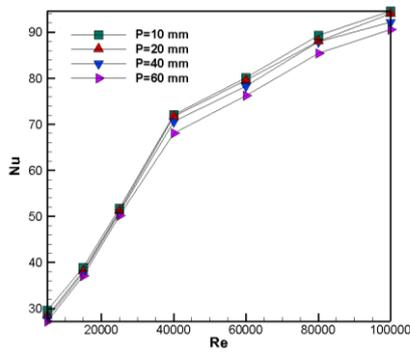
Fig. 7. Variation of Nusselt number with Reynolds number for various coil pitch
