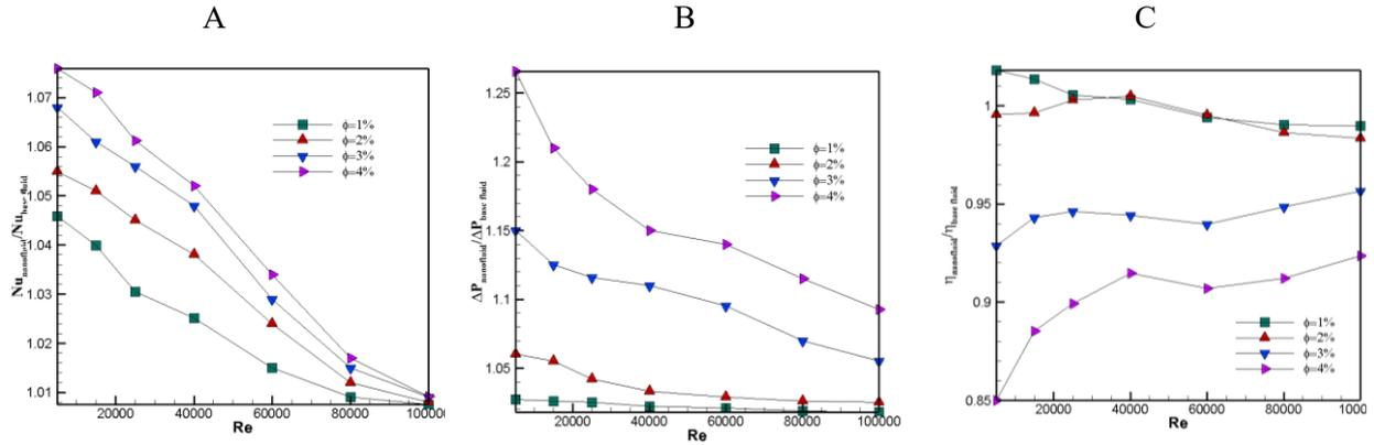
Fig. 9. A) Nanofluid Nusselt number to that of the base fluid ratio variation, B) Nanofluid pressure drop to that of base fluid ratio variation, C) Nanofluid performance evaluation criteria to that of the base fluid variation with Reynolds number for various water/aluminum oxide nanofluid nanoparticle volume fraction flowing inside the helical-coil tube for  $d = 9$  mm and  $D = 112$  mm.
