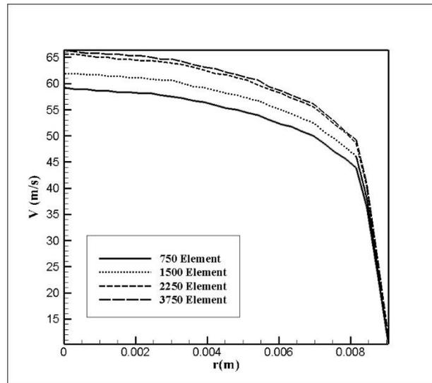
Fig. 3. Velocity distribution in cross section of straight tube with radius for various element numbers Fig. 4. Comparison between the results of present simulation for the coefficient of performance in the straight tube with the data of Elshafei et al. [29] at  $f=13.3$  Hz.
