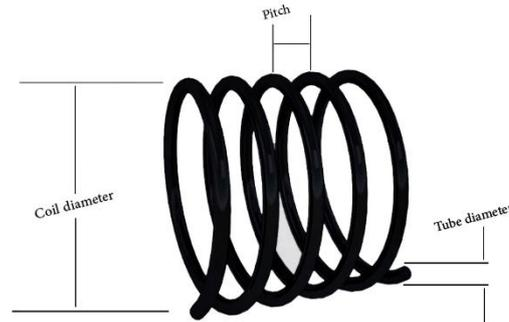
Fig. 1. Geometry of helical-coil tube
