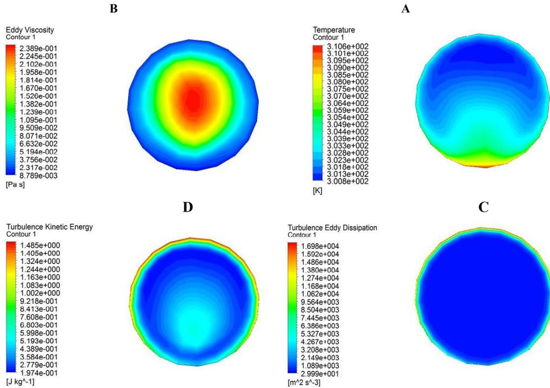
Fig. 6. Contour on the helical-coil tube exit. A) The temperature contour; B) The eddy viscosity; C) The eddy dissipation; and D) The turbulence kinetic energy
