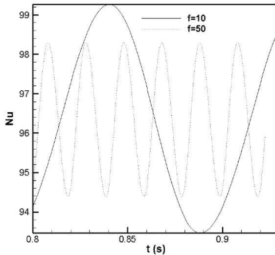
Fig. 11. Nusselt number variation with time for fluid flow inside the helical-coil tube with  $d = 9$  mm and  $D = 112$  mm for two frequencies of 10 Hz and 50 Hz
