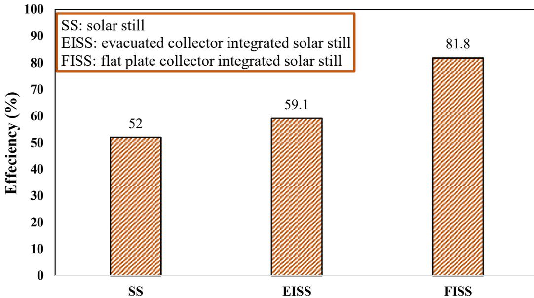
Fig. 13. Efficiency comparison between solar still and combined systems
