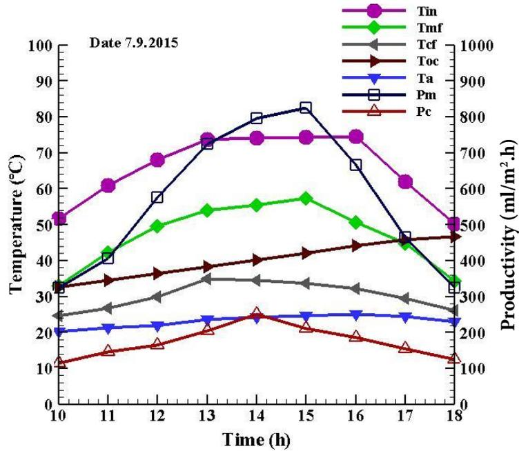
Fig. 9. Variations of temperature and productivity per hour in the experiment conducted on 7 August 2015
