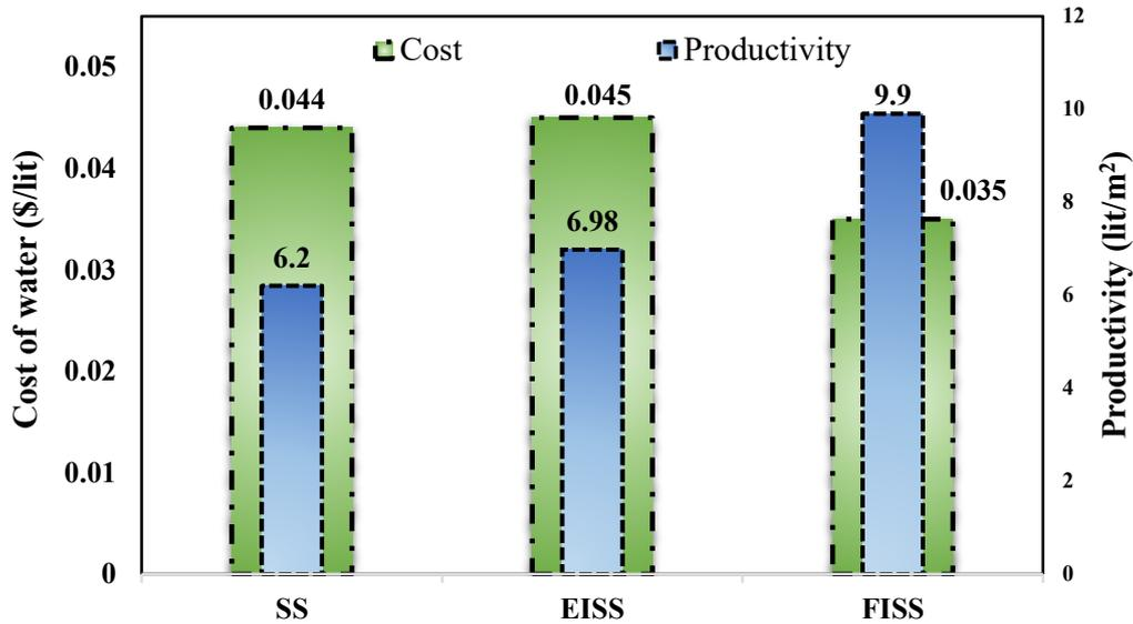
Fig. 15. Comparison of productivity and fresh water cost between combined systems and plain solar still
