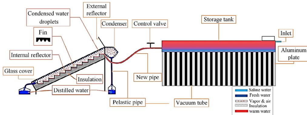
Fig. 1. Schematic view of the evacuated collector integrated solar still
