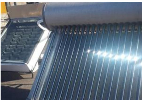
Fig. 3. A view of the evacuated collector integrated solar still
