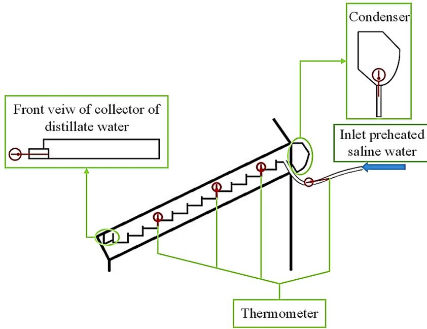
Fig. 5. Positioning of thermocouples
