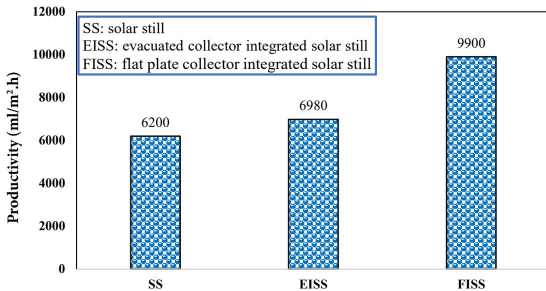
Fig. 14. Fresh water productivity comparison between solar still and combined systems
