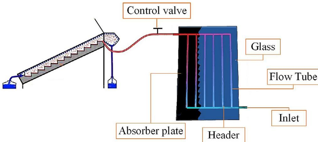
Fig. 2. Schematic view of the flat plate collector integrated solar still
