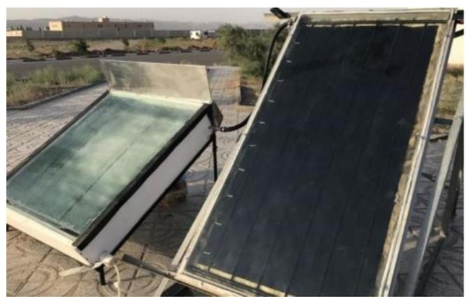
Fig. 4. A view of the flat plate collector integrated solar still
