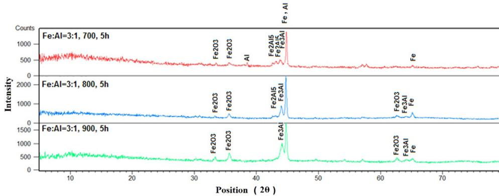
**Fig. 3. XRD results for the samples heat treated for 5 h at 700, 800 and 900°C containing the molar ratio of 3:1 of iron and aluminum.**
