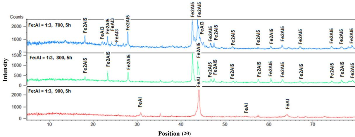
Fig. 7. XRD result for the samples heat treated for 5 h at 700, 800 and 900°C containing the molar ratio of 1:3 of iron and aluminum.
