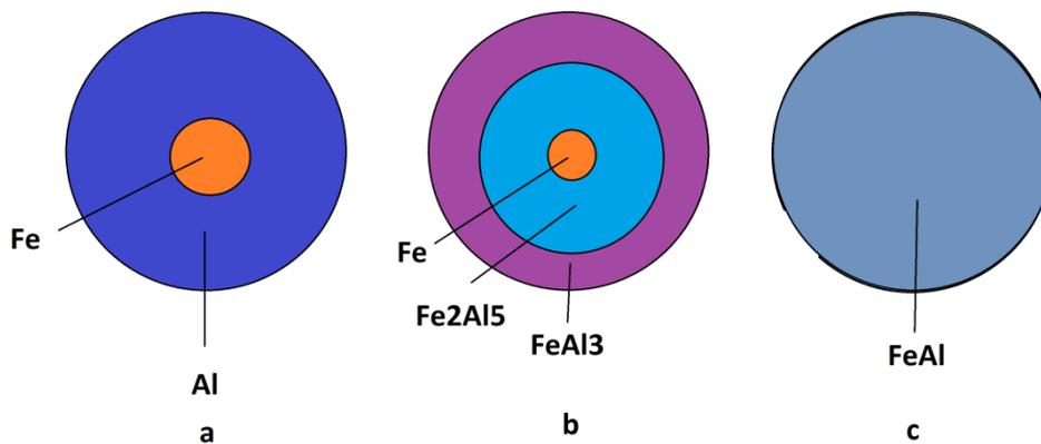
Fig. 8. Schematic trend of the reactions in Fe:Al=1:3 ratio.
