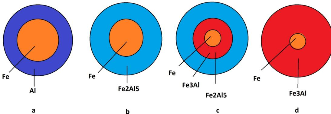
**Fig. 4. Schematic of the proposed mechanism in the ratio of 3:1 of iron and aluminum.**
