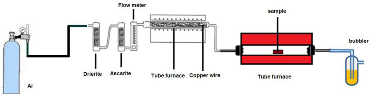
Fig. 1. The applied setup to prevent the oxidation.
