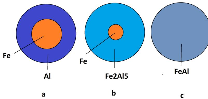
Fig. 6. Schematic trend of the reactions in Fe:Al=1:1 ratio.
