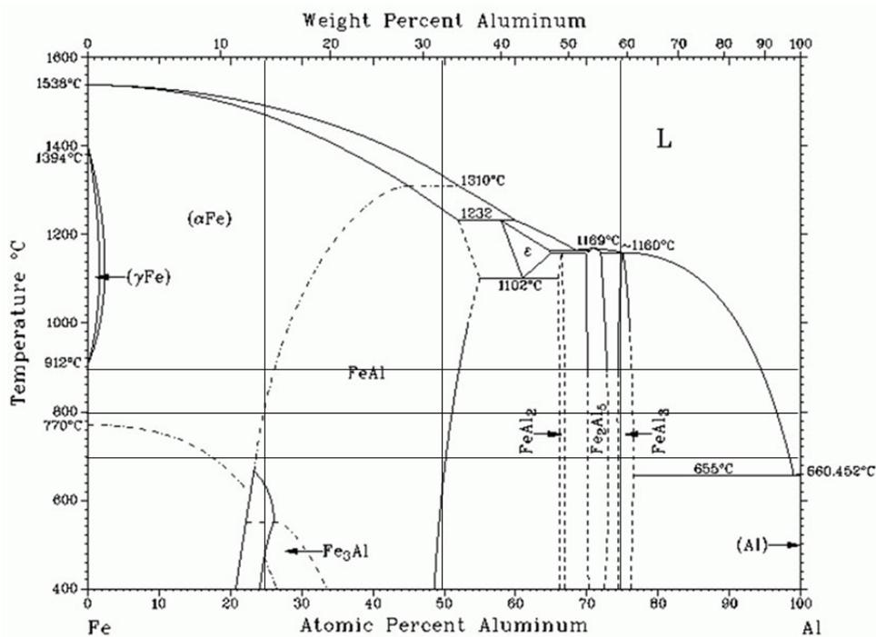
Fig. 2. Binary phase diagram of Fe and Al [16].
