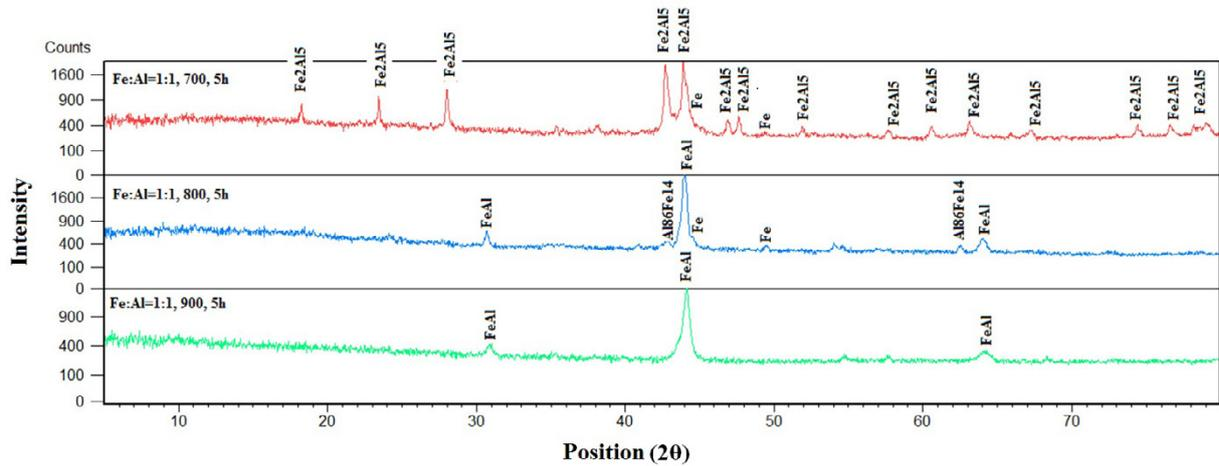
Fig. 5. XRD results for the samples heat treated for 5 h at 700, 800 and 900°C containing the molar ratio of 1:1 of iron and aluminum
