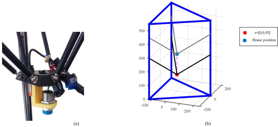
Fig. 12. Measurement setup (a) Connecting sensor to the MP's robot (b) The experiment measurement route
