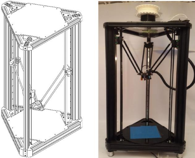
Fig. 1. The Delta 3D printer prototyped at the Amirkabir University of Technology (Tehran Polytechnic)
