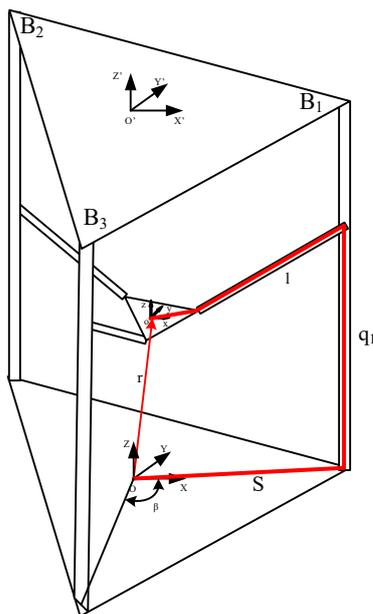
Fig. 2. Schematic of the robot with a vector loop
