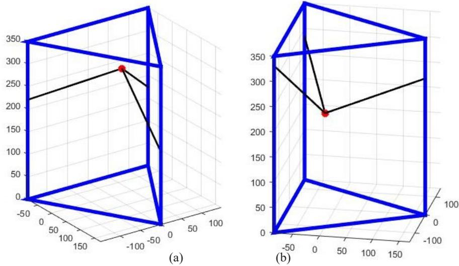
Fig. 3. Two possible configurations of the delta parallel robot to reach a position (a) Links are connected upward (b) Links are connected downward
