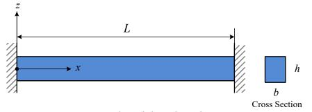
Fig. 1. A clamped-clamped microbeam.
