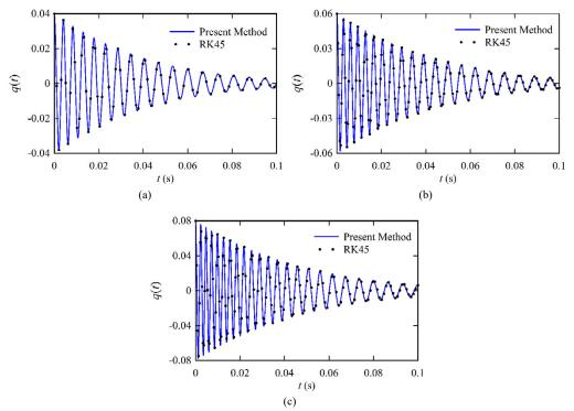
Fig. 4. Comparison between the responses of the clamped-clamped microbeam obtained by the first order of the new method and the numerical method for nondimensional vibration amplitudes of: (a)  $a_0 = 0.04$  (b)  $a_0 = 0.06$  (c)  $a_0 = 0.08$ .
