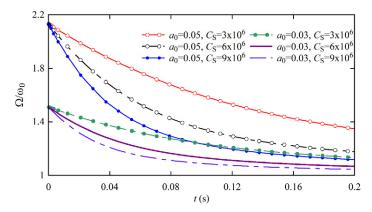
Fig. 5. Variation of the frequency ratio,  $\Omega/\omega_0$ , versus time for various values of the microbeam structural damping,  $C_s$ .
