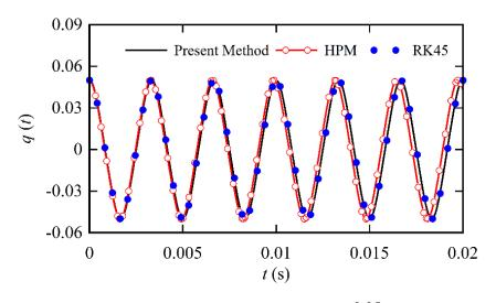
Fig. 2. Comparison among the responses of the clamped-clamped microbeam for  $a_0 = 0.05$  obtained by the new method, HPM and the numerical method
