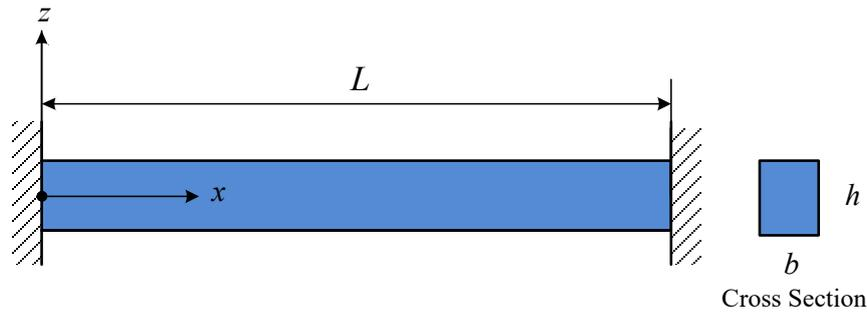
Fig. 1. A clamped-clamped microbeam.
