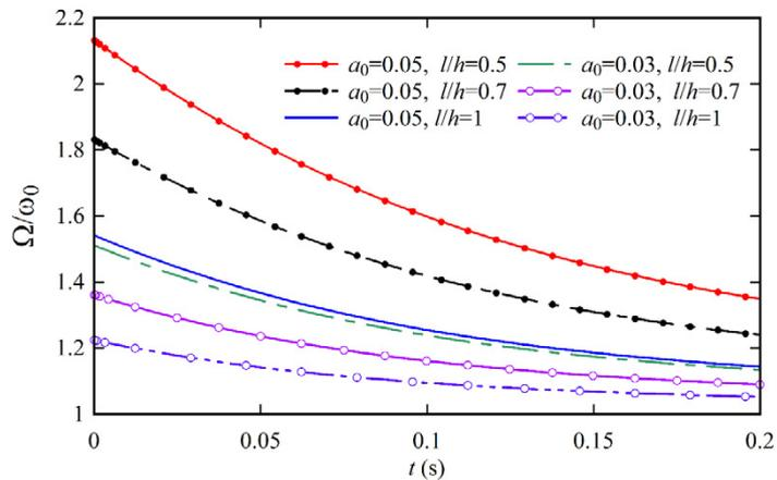
Fig. 6. Variation of the frequency ratio,  $\Omega/\omega_0$ , versus time for various values of the microbeam material length scale parameter,  $l$  .
