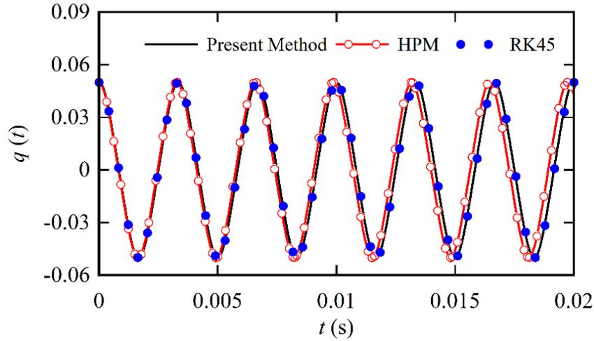
Fig. 2. Comparison among the responses of the clamped-clamped microbeam for  $\alpha_0=0.05$  obtained by the new method, HPM and the numerical method
