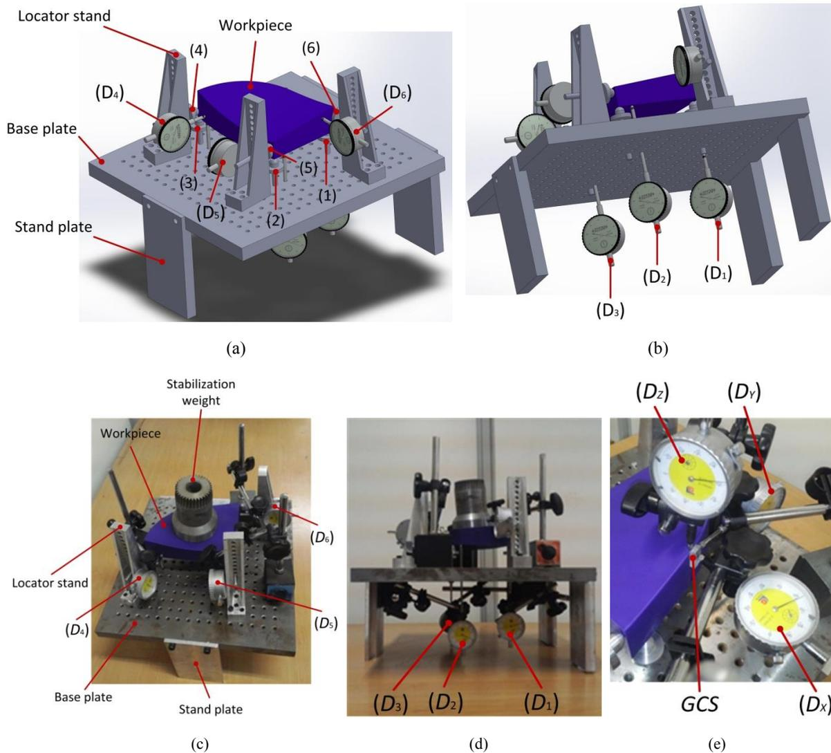
Fig. 4. The experimental setup designed for the second case study (a) and (b) setup model (c) and (d) the fabricated setup (e) experimental setup for measurement of workpiece locating error  $\{\Delta q\}$  at Global Coordinate System (GCS).
