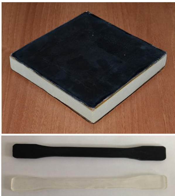
Fig. 1. . Sandwich plate sample and tensile test samples
