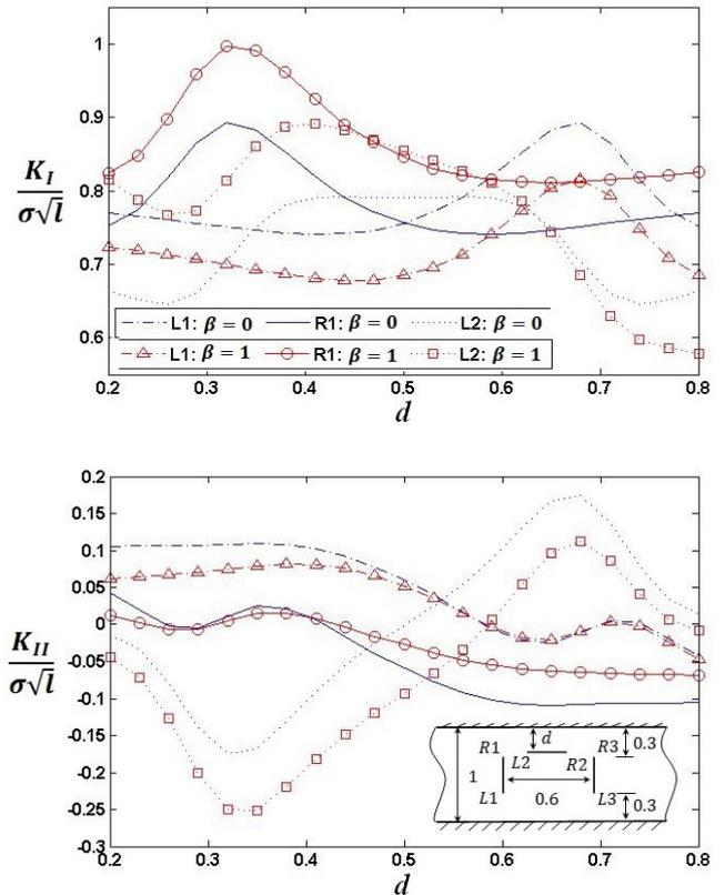
Fig. 6. SIFs for a variable location horizontal and two fixed vertical cracks
