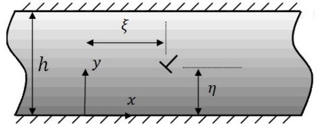
Fig. 1. Schematic view of a FG layer weakened by an edge dislocation
