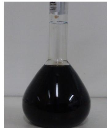
**Fig. 8. Photograph of graphene oxide nanoplatelets nanofluid GO3, after 440 days**
