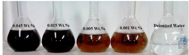
Fig. 4. The image of nanofluid samples with different weight percentages
