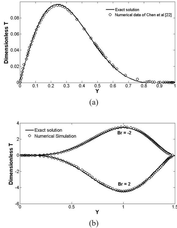
**Fig. 2. Comparison of presented exact solution for dimensionless temperature distribution with (a) numerical results of Chen et al. [22] at  $Br=0$  and (b) numerical simulations at  $Br=2, -2$**
