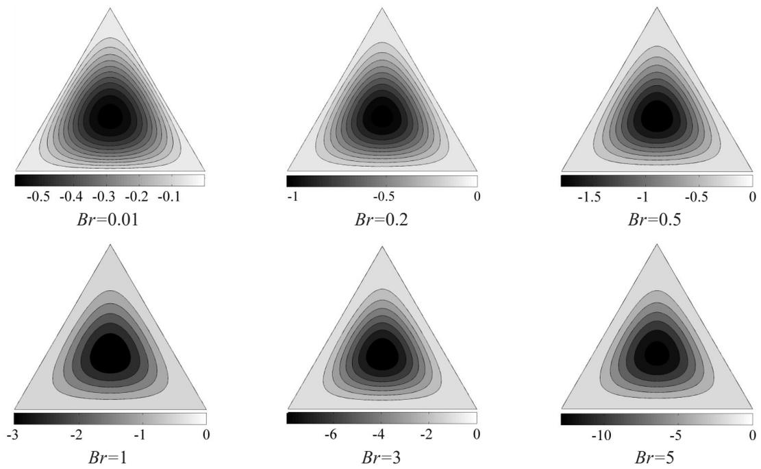
**Fig. 4. Dimensionless contours of temperature for flow in triangular ducts (Heating).**
