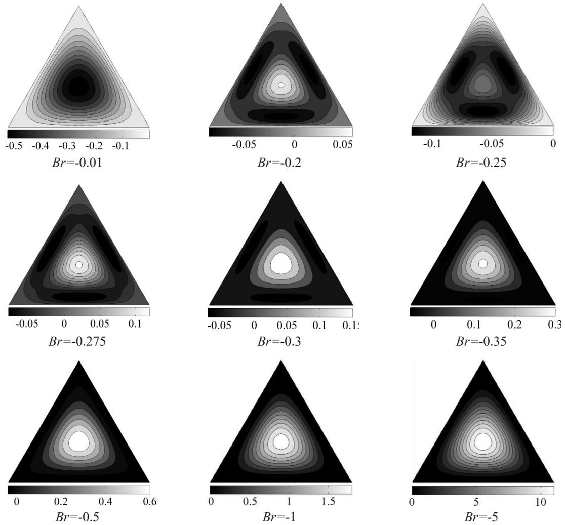
**Fig. 3. Dimensionless contours of temperature for flow in triangular ducts (Cooling).**
