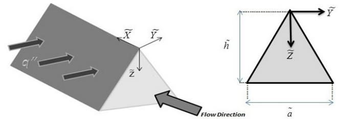
Fig. 1. The geometry of duct in current study
