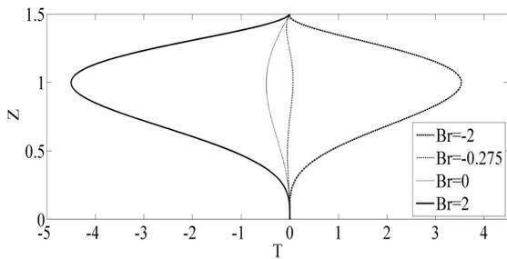
Fig. 6. Profile of absolute value of dimensionless temperature along the symmetry axis of cross section
