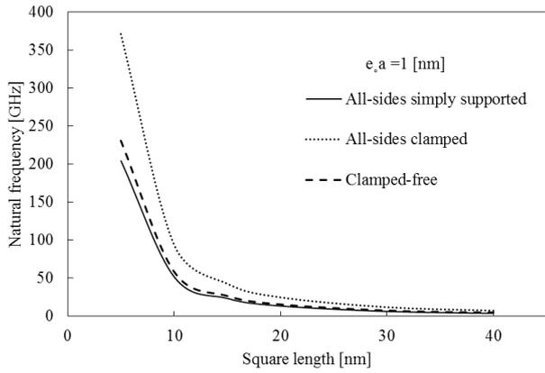
**Fig. 6.** Variations of fundamental natural frequencies with length of the square nano-plate considering  $e_0 a = 1$  for different boundary conditions
