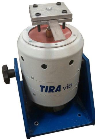
**Fig. 8. Cantilever energy harvester that is mounted on the shaker**
