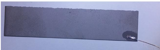
**Fig. 7. Soldering the wires to the piezoelectric layer**
