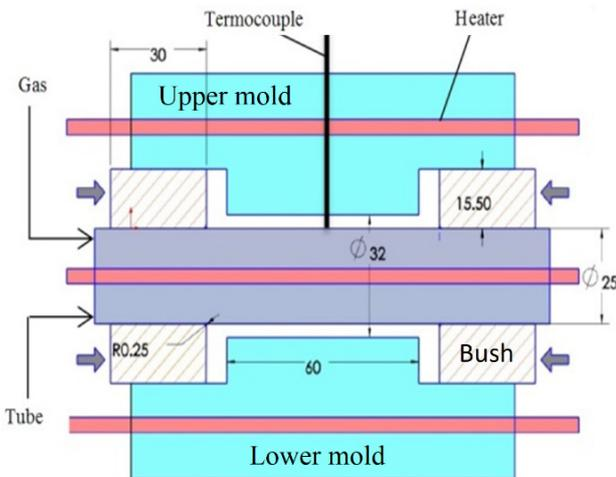
**Fig. 2. Schematic of mold set designed**
