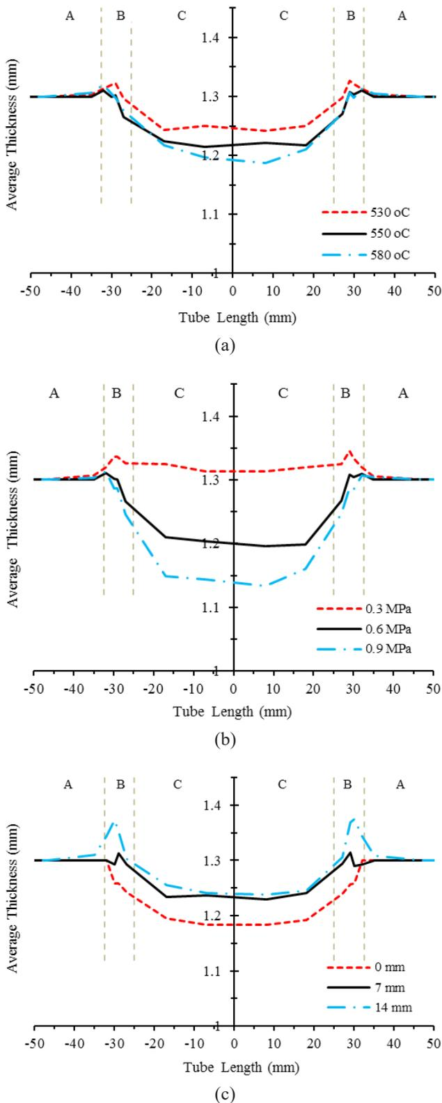
Fig. 9. The average thickness distribution at various a) temperatures b) pressures, and c) axial feeds
