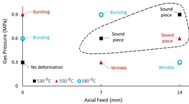
**Fig. 7. The HMGF process parameters window**
