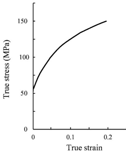
**Fig. 1. True stress-strain curves of AA6063**
