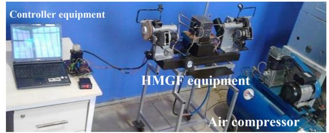
**Fig. 3. The HMGF process equipment**
