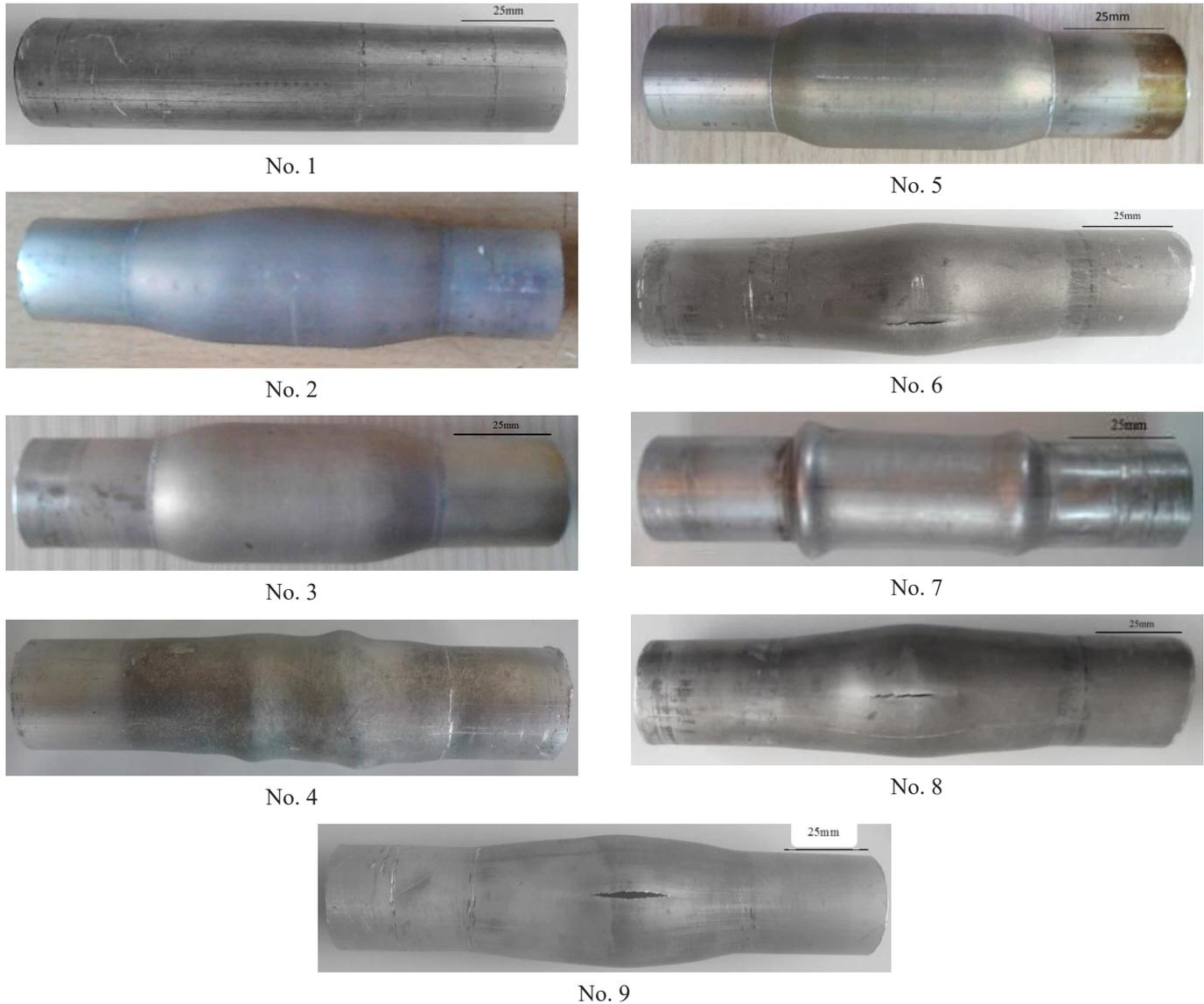
Fig. 6. The specimens after forming process
