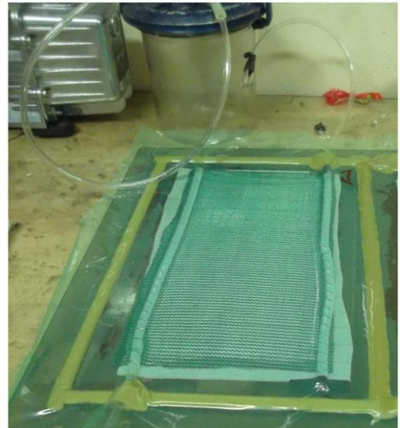
Fig. 2. VARTM process setup to construct FMLs face sheets
