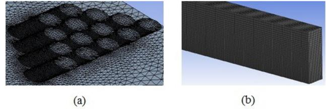
Fig. 3. Computational grid for fan shape multi-hole, a) second block, b) first block.
