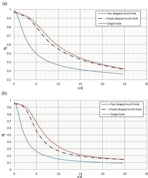
Fig. 12. Centerline film cooling effectiveness, a)  $M = 0.6$  and b)  $M=1.25$ .
