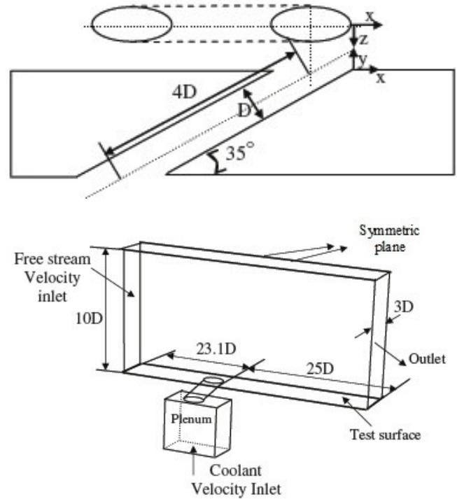
Fig. 1. Computational domain and boundary conditions for a single hole [7].
