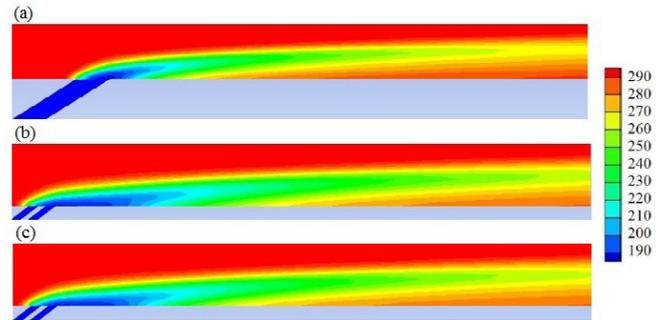
Fig. 8. Centerline plane temperature contours for  $M=1.25$ , a) single hole, b) fan shape holes, c) hook shape holes.
