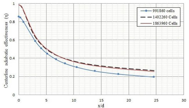
Fig. 4. Grid sensitivity for a single cylindrical hole,  $M = 0.6$ .
