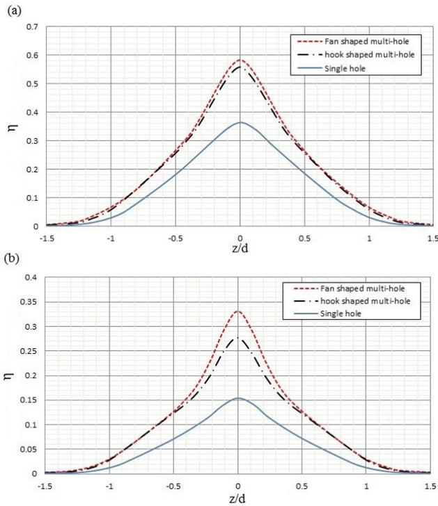
Fig. 13. Spanwise film cooling effectiveness at  $x/D = 10$ , a)  $M = 0.6$ , b)  $M = 1.25$
