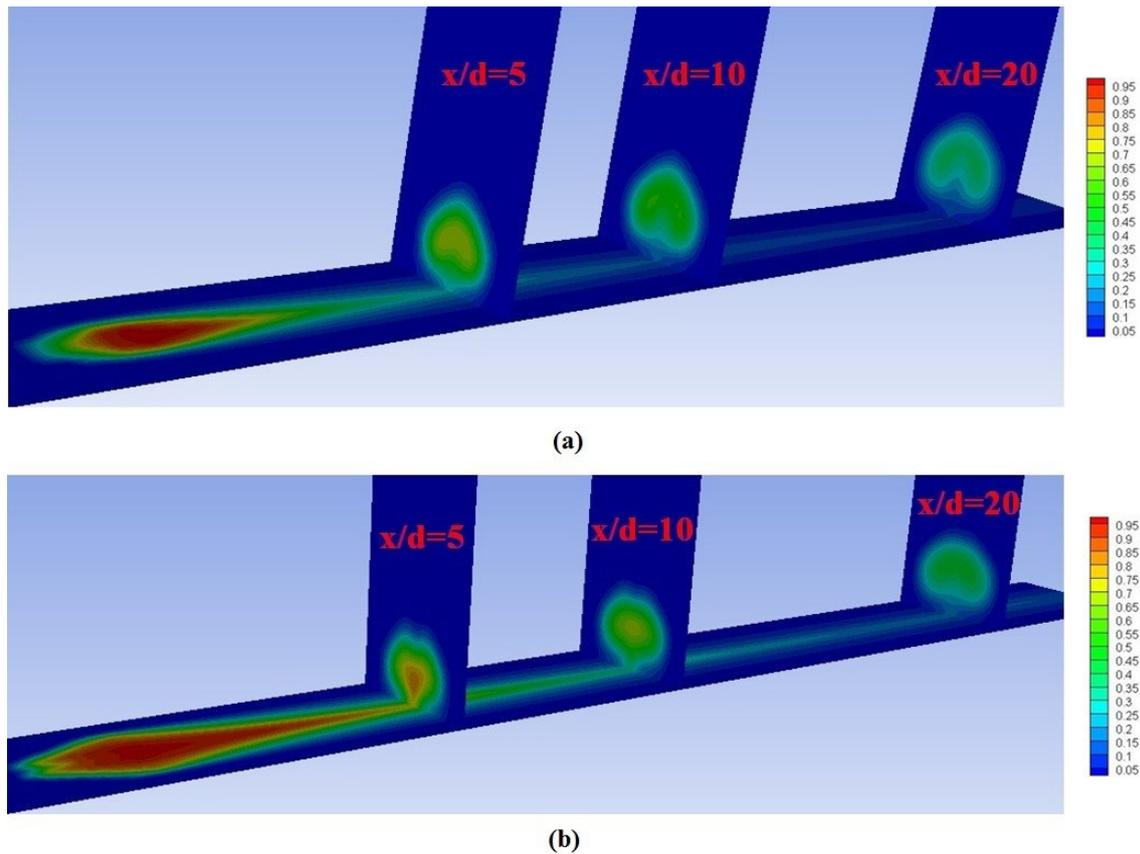
Fig. 9. Contours of adiabatic effectiveness change with non-dimensional temperature at different streamwise locations at  $M=1.25$ , a) single hole, b) fan shape holes.
