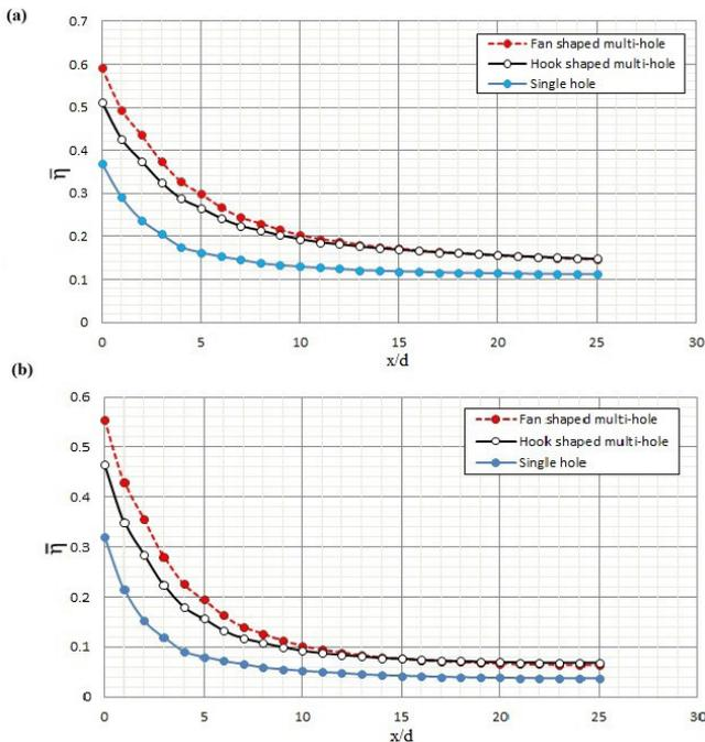
Fig. 14. Laterally averaged film cooling effectiveness, a)  $M = 0.6$ , b)  $M = 1.25$ .
