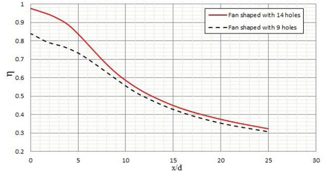
Fig. 15. Comparison of centerline adiabatic effectiveness of fan shaped multi-hole at  $M = 0.6$  with 9 and 14 holes.
