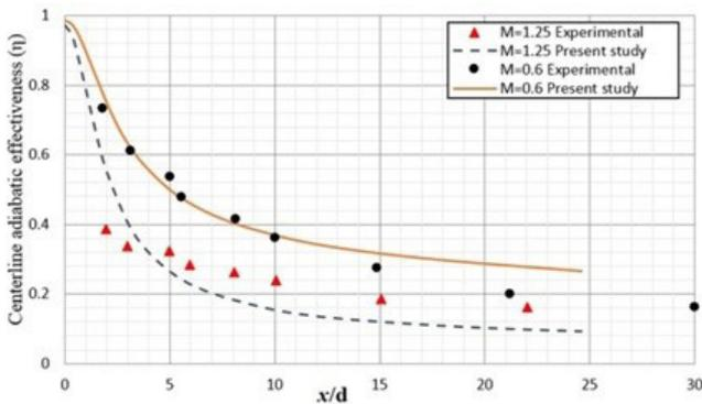
Fig. 6. Comparison of the centerline effectiveness with the experimental data [23].
