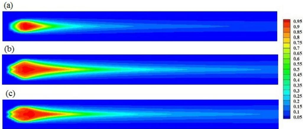
Fig. 11. Contours of film cooling effectiveness for  $M=1.25$ , a) single hole, b) fan shape holes, c) hook shape holes.
