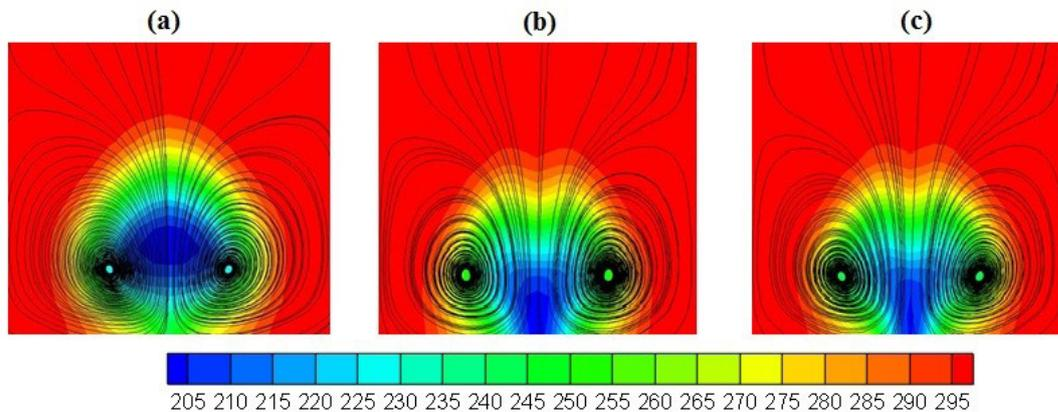
Fig. 10. Velocity contours along with streamlines change with Velocity contours along with temperature,  $M = 1.25$ ,  $x/d = 3$ , a) single hole, b) fan shape holes, c) hook shape holes.
