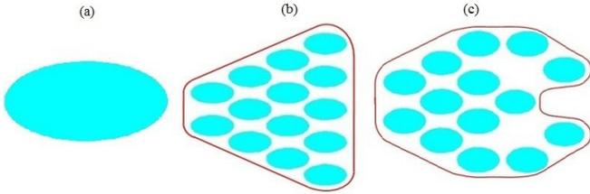
Fig. 2. Film cooling configurations, a) single hole, b) multi-hole with fan shape, c) multi-hole with hook shape.
