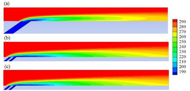
Fig. 7. Centerline plane temperature contours for  $M=0.6$ , a) single hole, b) fan shape holes, c) hook shape holes.
