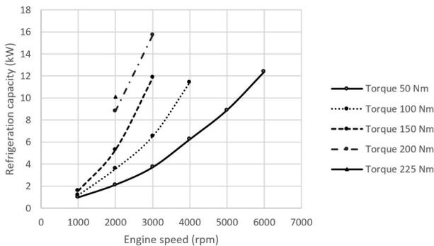
Fig. 18. Generated refrigeration capacities by system with refrigerant R1234yf in different speeds and torques of gasoline engine
