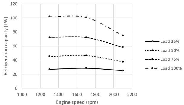
**Fig. 15. Generated refrigeration capacities by system with refrigerant R290 in different speeds and loads of diesel engine**
