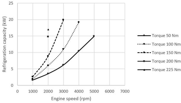
Fig. 16. Generated refrigeration capacities by system with refrigerant R600 in different speeds and torques of gasoline engine
