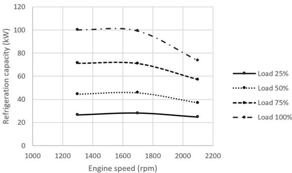
**Fig. 11. Generated refrigeration capacities by system with refrigerant R134a in different speeds and loads of diesel engine**
