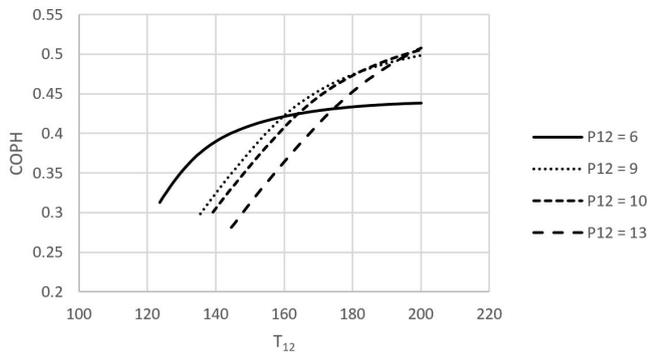
**Fig. 4. COPH versus temperature and pressure for R134a refrigerant. Optimum value for COPH is at  $P_{12} = 9$  MPa,  $T_{12} = 180$  °C, ( $COPH = 0.4742 - COPW = 12.55 - COP = 4.098$ )**
