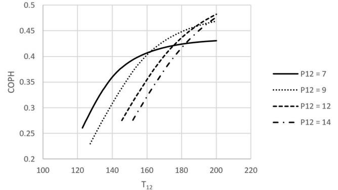
**Fig. 6. COPH versus temperature and pressure for R600. Optimum value for COPH is at  $P_{12} = 12$  MPa,  $T_{12} = 200$  °C, ( $COPH = 0.4824 - COPW = 8.142 - COP = 3.997$ )**
