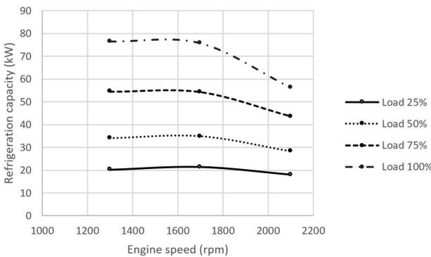
Fig. 19. Generated refrigeration capacities by system with refrigerant R1234yf in different speeds and loads of diesel engine
