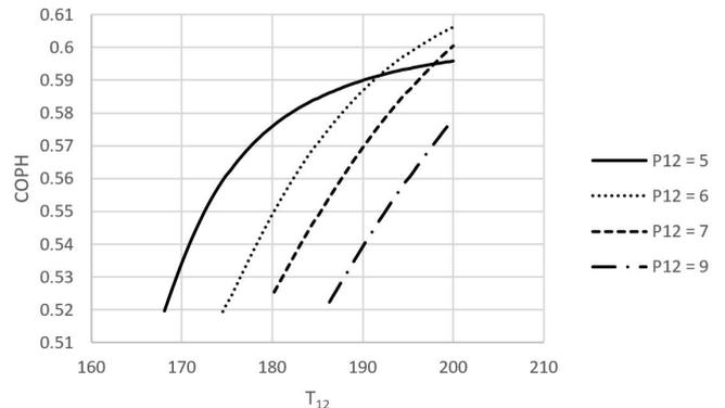
**Fig. 7. COPH versus temperature and pressure for R290. Optimum value for COPH is at  $P_{12} = 6$  MPa,  $T_{12} = 200$  °C, ( $COPH = 0.6062 - COPW = 24.84 - COP = 4.32$ )**
