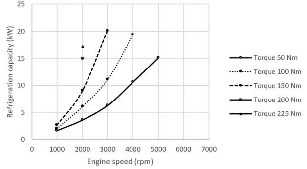
**Fig. 12. Generated refrigeration capacities by system with refrigerant R245fa in different speeds and torques of gasoline engine**
