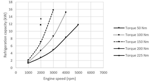
**Fig. 14. Generated refrigeration capacities by system with refrigerant R290 in different speeds and torques of gasoline engine**
