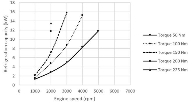
Fig. 20. Generated refrigeration capacities by system with refrigerant R1270 in different speeds and torques of gasoline engine
