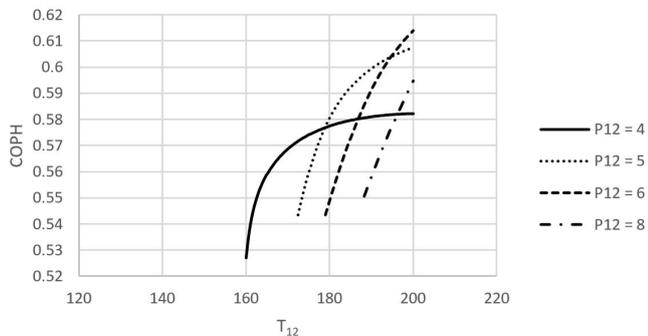
**Fig. 5. COPH versus temperature and pressure for R245fa. Optimum value for COPH is at  $P_{12} = 6$  MPa,  $T_{12} = 200$  °C, ( $COPH = 0.614 - COPW = 29.16 - COP = 4.339$ )**
