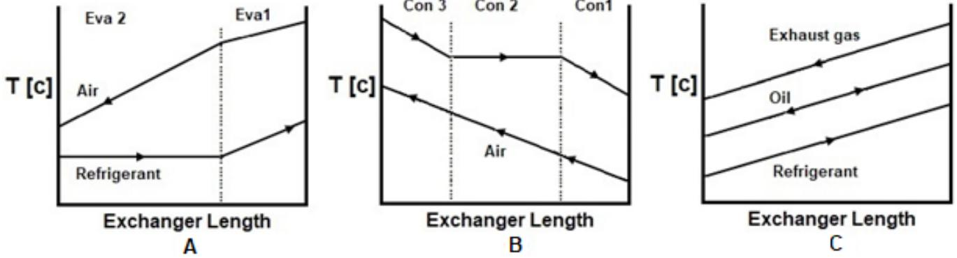
Fig. 3. (A) Evaporator, (B) Condenser, (C) heat exchanger of the exhaust gas
