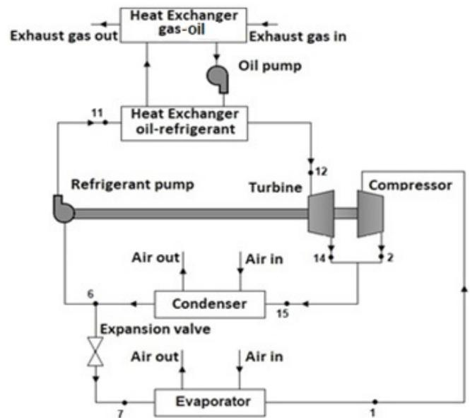
Fig. 1. Schematic scheme of refrigeration system.
