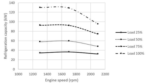
**Fig. 13. Generated refrigeration capacities by system with refrigerant R245fa in different speeds and loads of diesel engine**
