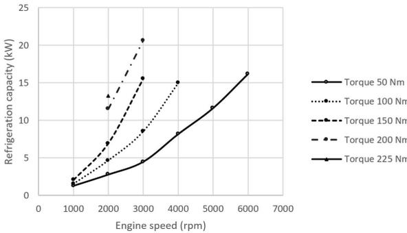
**Fig. 10. Generated refrigeration capacities by system with refrigerant R134a in different speeds and torques of gasoline engine**
