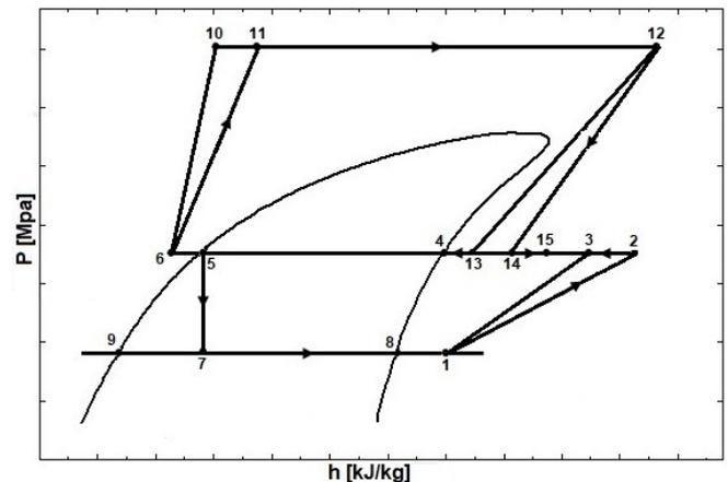
Fig. 2. Schematic display of the refrigeration system in  $P-h$  diagram for R245fa refrigerant
