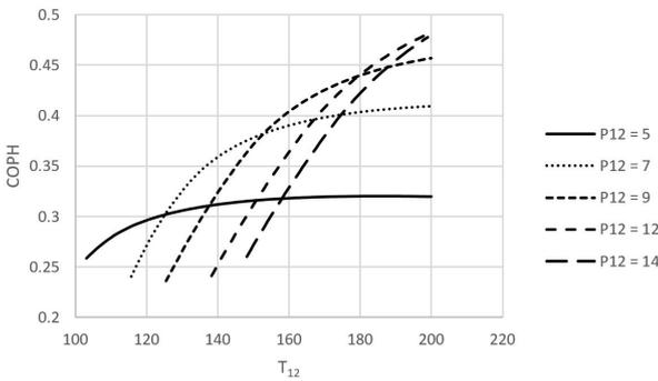
**Fig. 9. COPH versus temperature and pressure for R1270. Optimum value for COPH is at  $P_{12} = 12$  MPa,  $T_{12} = 200$  °C, ( $COPH = 0.4819 - COPW = 8.365 - COP = 3.971$ )**
