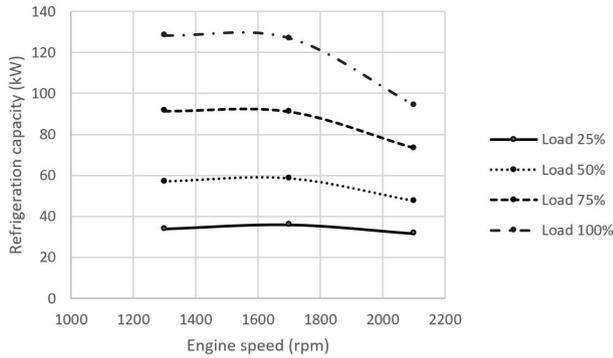
Fig. 17. Generated refrigeration capacities by system with refrigerant R600 in different speeds and loads of diesel engine
