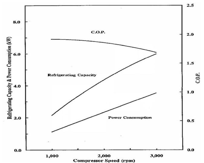
Fig. 22. SD6V12 performance diagram [33]
