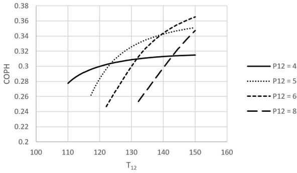
**Fig. 8. COPH versus temperature and pressure for R1234yf. Optimum value for COPH is at  $P_{12} = 6$  MPa,  $T_{12} = 150$  °C, ( $COPH = 0.3652 - COPW = 11.59 - COP = 3.903$ )**
