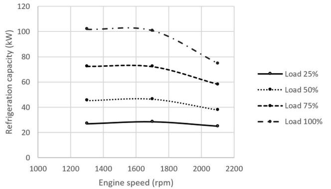
Fig. 21. Generated refrigeration capacities by system with refrigerant R1270 in different speeds and loads of diesel engine
