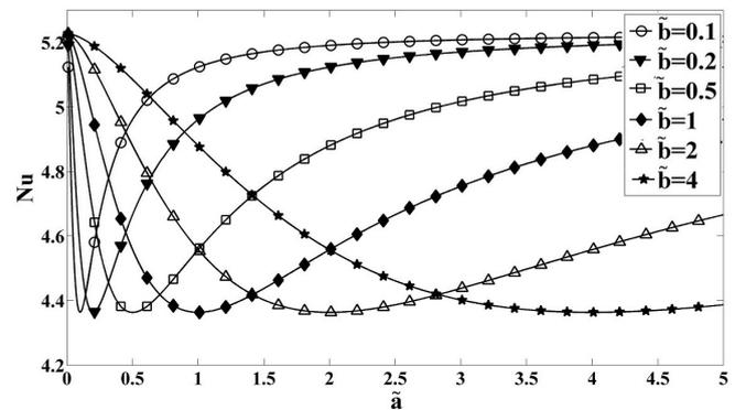
Fig. 5. Diagrams of Nusselt number in terms of the major and minor axes of the elliptical cross-section
