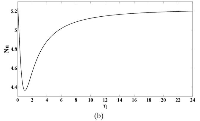
Fig. 4. Diagrams of the (a) absolute value of dimensionless temperature at the center of cross section and (b) Nusselt number versus the aspect ratio
