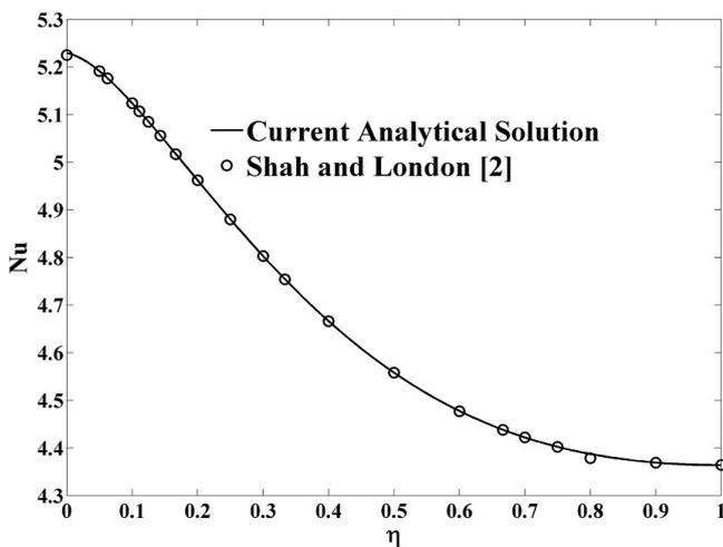
Fig. 2. The comparison of Nusselt number versus aspect ratio ( $\eta$ ) for forced convection heat transfer in elliptical pipes between the current analytical solution (Eq. (28)) and study of Shah and London [2]
