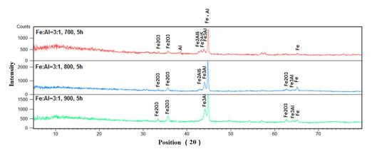
Fig. 3. XRD results for the samples heat treated for 5 h at 700, 800 and 900°C containing the molar ratio of 3:1 of iron and aluminum.
