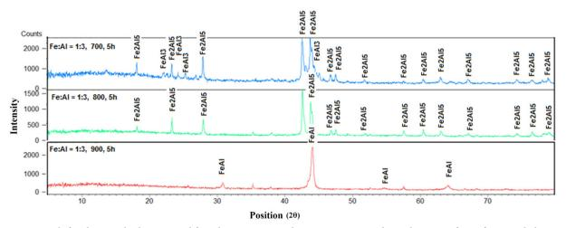
Fig. 7. XRD result for the samples heat treated for 5 h at 700, 800 and 900°C containing the molar ratio of 1:3 of iron and aluminum.
