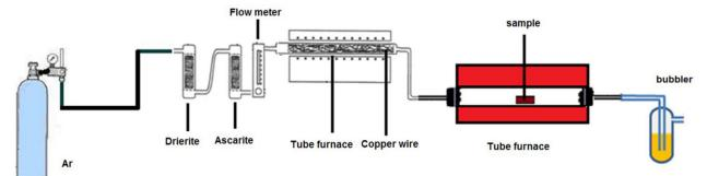
Fig. 1. The applied setup to prevent the oxidation.
