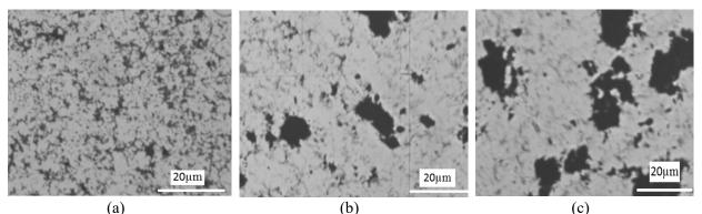
Fig. 9. OM images of the samples with the molar ratios of a) 3:1, b) 1:1 and c) 1:3 of iron and aluminum heat treated for 5 h 900°C.
