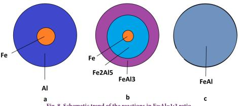
Fig. 8. Schematic trend of the reactions in Fe:Al=1:3 ratio.
