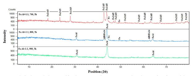
Fig. 5. XRD results for the samples heat treated for 5 h at 700, 800 and 900°C containing the molar ratio of 1:1 of iron and aluminum
